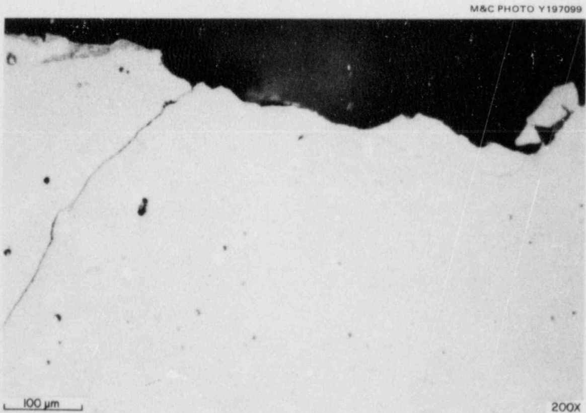
Fig. 6.11. Detail of location 1 in Fig. 6.10 showing fracture path in type 309 cladding following patches of ferrite.
