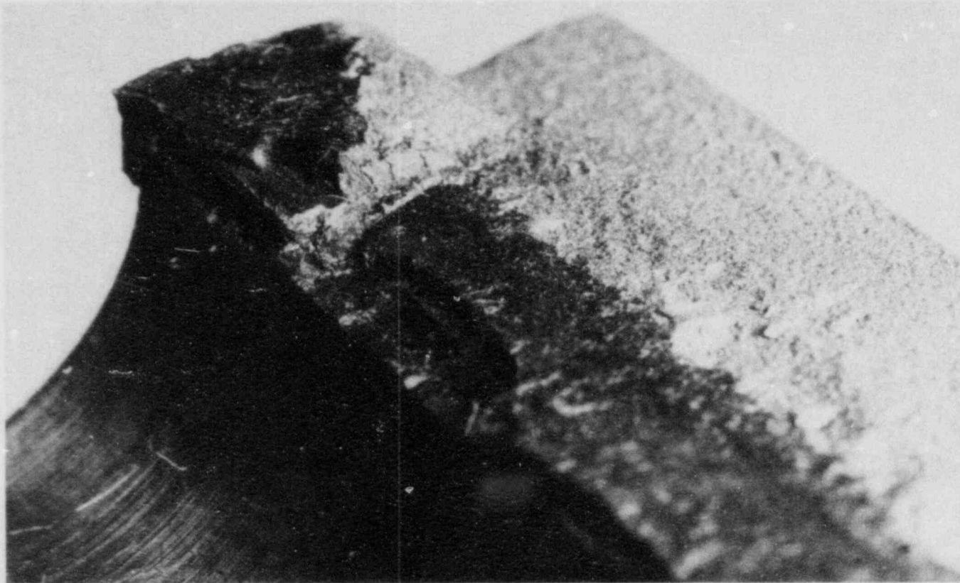
Fig. 5.12. Broken half of mockup showing flaw path of H_2 -charged juxtaposed EB welds.
