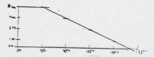
Pot life stated above for unthinned coatings are the recommended times and should be utilized as a guideline for coatings usage times, however, actual pot life may be longer. For unthinned coatings or coatings thinned 50% or less, actual pot life is determined by applicability of the coating.
