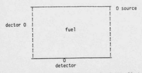
This arrangement allows the detectors to "see" the effects of fuel addition without being shadowed by source neutrons.
