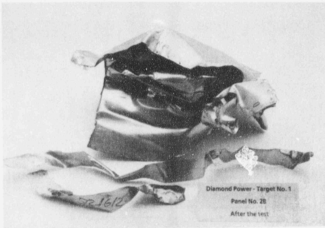
Figure 4 RMI Foil Debris From Siemens KWU Steam Blowdown No. 1 Test (5/31/95)
