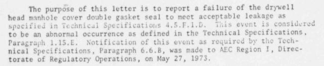
While attempting to pressurize the double gasket seal on the drywell head manhole cover, significant pressure decay was observed between the gaskets. A check of the manhole cover plate with leak teck showed that there was a significant amount of leakage through the outer gasket. No attempt was made to determine whether the inside gasket was leak tight. The allowable leakage for a penetration is 10% of Lt(20) or 19.9 SCFH.
