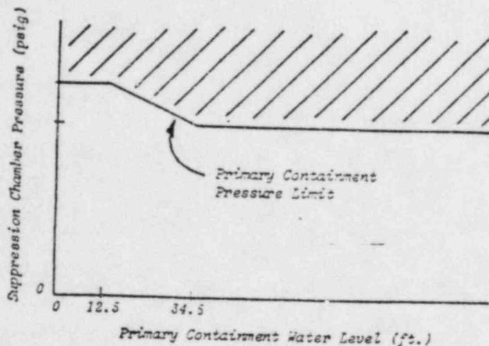
PC/P-7 If suppression chamber pressure exceeds the Primary Containment Pressure Limit, vent the primary containment in accordance with [procedure for containment venting] to reduce and maintain pressure below the Primary Containment Pressure Limit.
