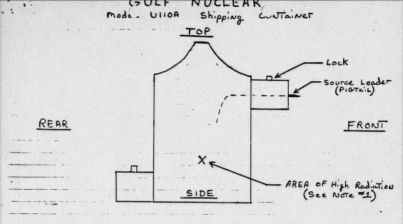
NOTE #1: AREA OF HOT Spot is approx. 12" in diameter on surface of shipping container. Beam spread equaled about 3" at a distance of 3' from the container.
