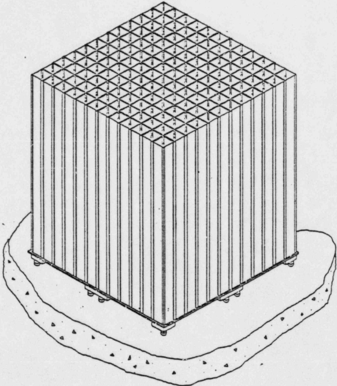
Figure 2. Fuel Storage Rack Assembly in Region 2
