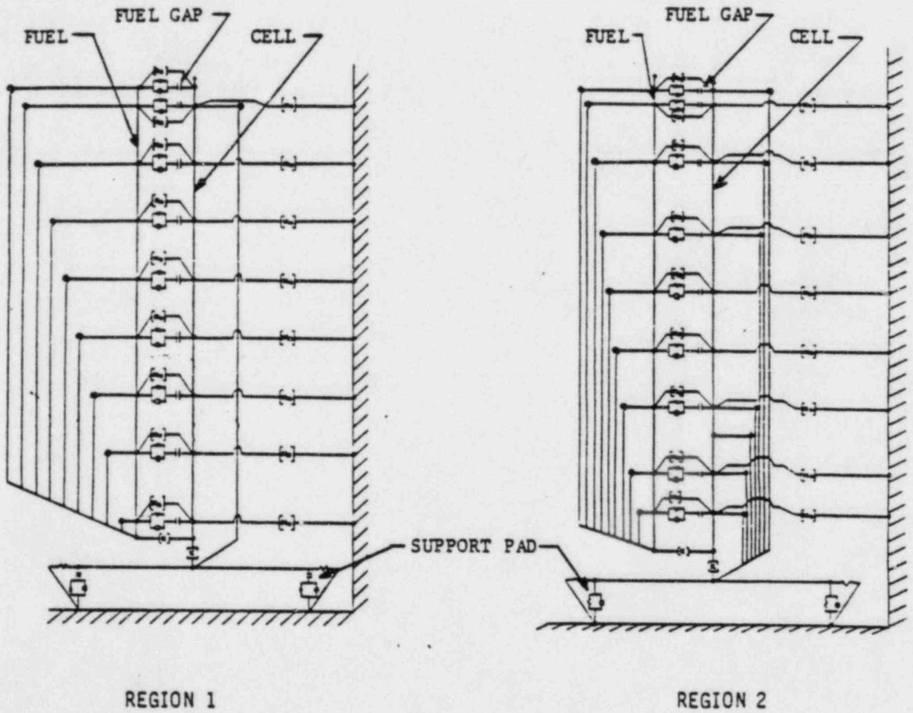
Figure 3. Two-Dimensional Nonlinear Model
