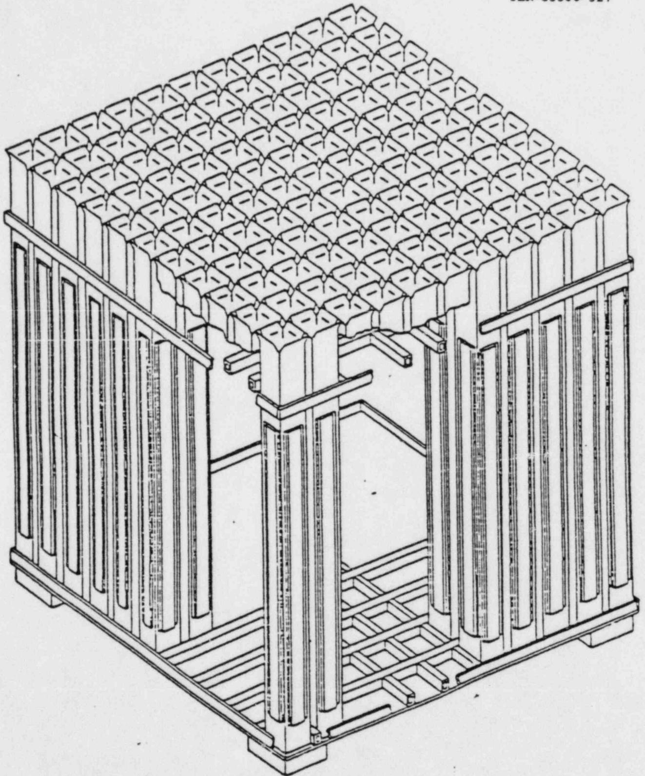
Figure 1. Fuel Storage Rack Assembly in Region 1
