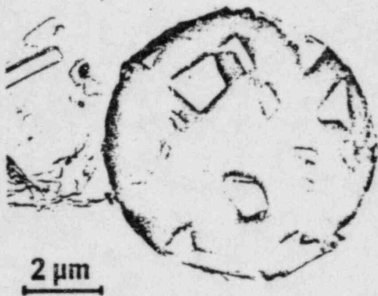
Fig. 3. Transmission electron micrograph of a replica of a fly ash sphere showing abundant mullite needles. The association of crystals-within-sphere is retained by the replica; the original glassy material is dissolved during the replication process, but mullite is insoluble in HF. (Photos courtesy of G. A. Waits, D. S. McKay, and D. L. Gibbon, Lyndon B. Johnson Space Center, Houston, Texas.)
