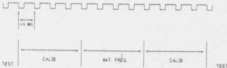
TYPICAL TEST RECORD - FORCED BALANCE ACCELEROMETER (FBA)
