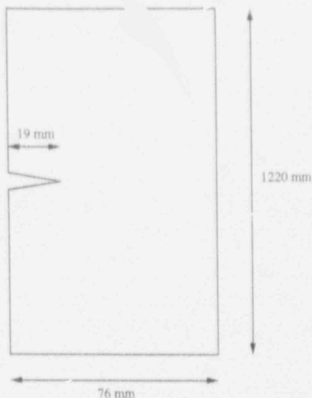
Figure G.3 Schematic of the 2-D SEN geometry associated with central, GPS portion of biaxial specimen
