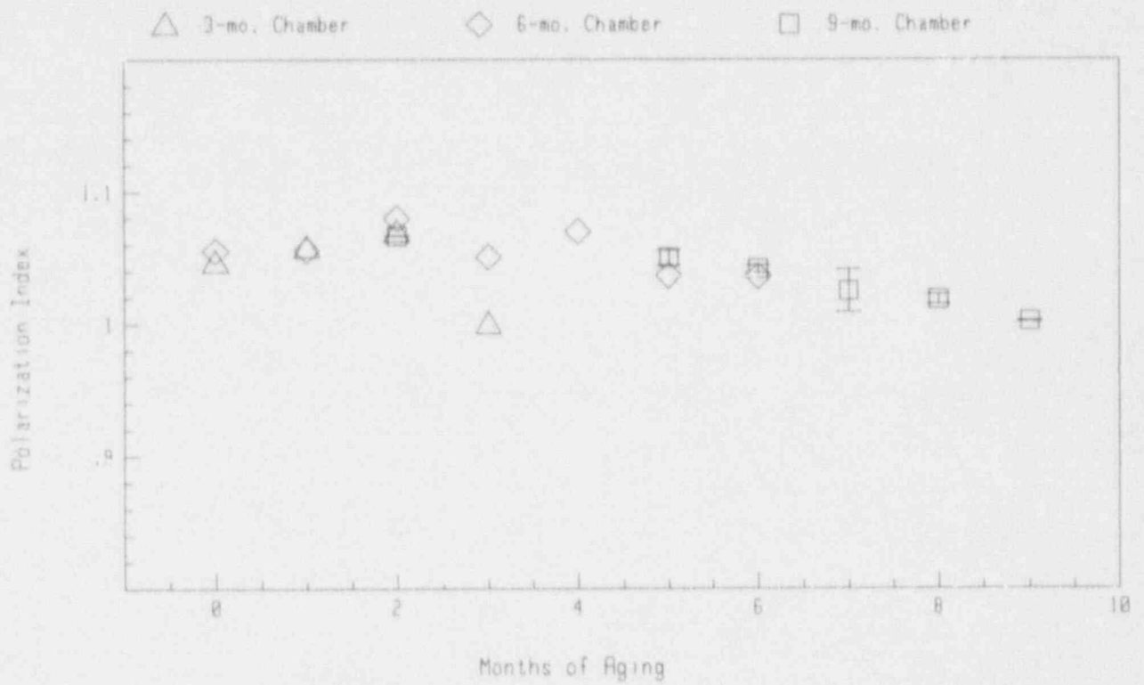
Figure C-19 250 V PI (5 min/30 s) of Polysset Jacket During Aging
