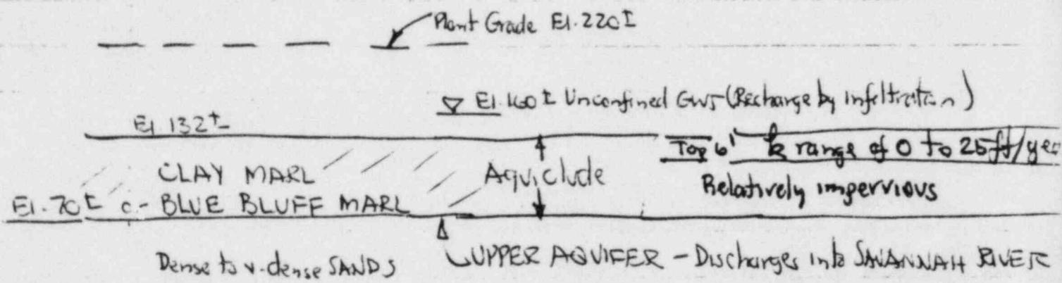
\* pg. 2.5.4-10) Power block structures designed to GROUNDWATER El. 160
