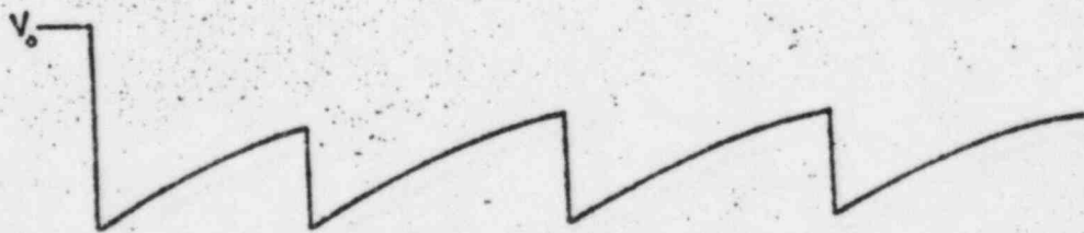
Figure 14-3d: Signal at Point "A" of Figure 14-3a when Circuit Designed for Current Operation
