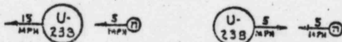
Figure 10-31: Conditions Which Will Result in Neutron Absorption in A Fictitious U-238 Absorption Resonance at 10 MPH
