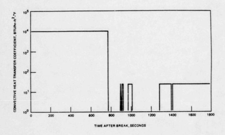
Title: Frul Port Comertine Heat Transfer Coefficient 15. Time Often Break (Small Break Model) Main Steam Line Break Outsiles Containment, Failure of Channel A DC Source)
