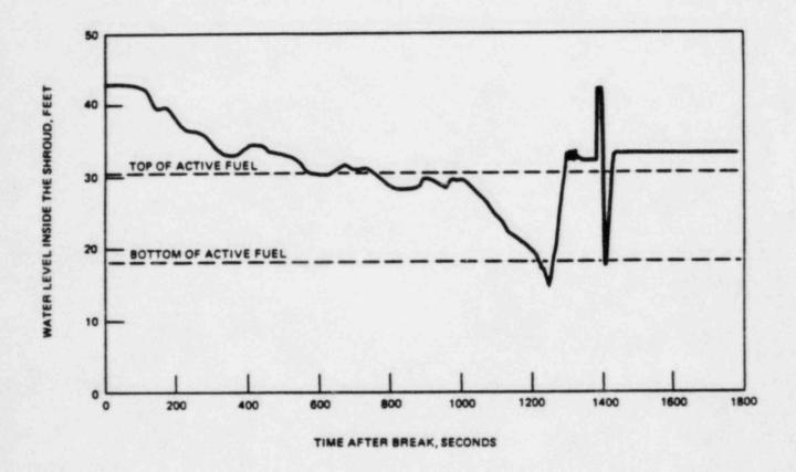
Title: Water level driede Shoul vs Time after Break Orthide (Maximum Main Steam Line Break Orthide Containment, Failure of Channel ADC Sommer)
