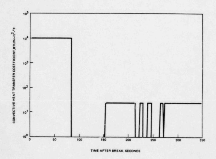
Tille: Ful Rod Connective Heat Transfer Coefficient 15. Time Often beach (Maximum Main Steam Line Break Shaile Containment, Failure of Chunel A DC Source)
