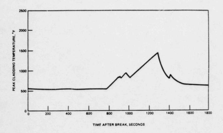
Title: Peak Cladling Temperature vs Time after Break (Small Brack Model) (Maximum Main Steam Line Break Outside Containment, Failure of Channel A DC Somee)
