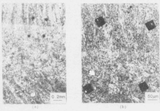
Figure 5 (a) Typical fusion line region of two weld bead runs within WF70 weldment showing change of microscructure across fusion line; (b) enlarged view of region of (a) sampled with microhardness indents
