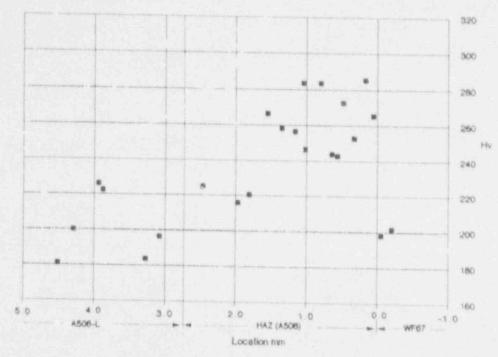
Figure 7 Microhardness results for indents in Fig. 6 in graph form. The abscissa is distance from fusion boundary parallel to straight line through set of indents
