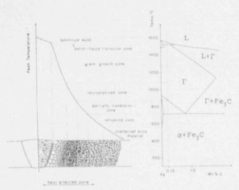
Figure 2 Schemati: diagram of various subzones of typical HAZ (from Ref. 2)
