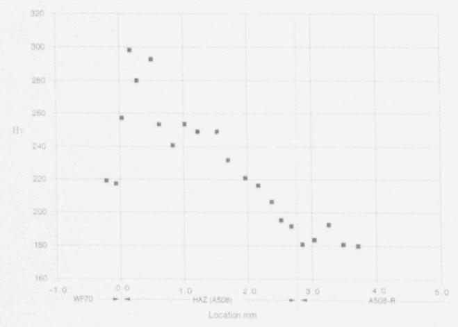
Figure 12 Results from microhardness indents in Fig. 11. Abscissa shows distance of indent from fusion boundary parallel to straight line through measurements group
