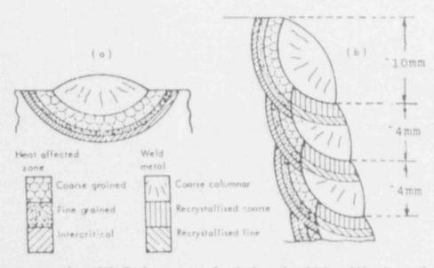
Figure 3 Schematic comparison of HAZ microstructure for single- and multiple-weld bead runs (from Ref. 2)
