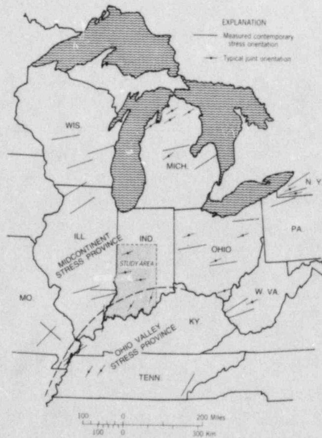
Figure 16. Map of part of the northeastern United States showing measured stress orientations and selected regional joints (adapted from Engelder, 1982).
