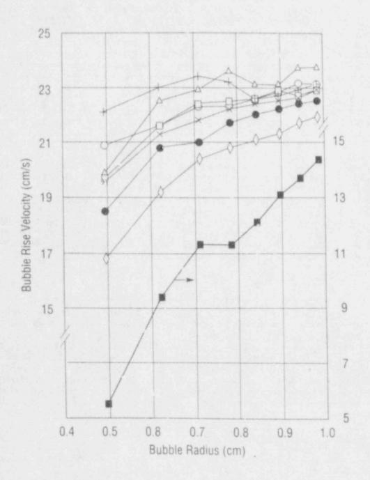
Figure 10. Measured bubble rise velocities: +-Water, O-Acetone, △-R11, □-Hexane, X-10 cs. Silicone Oil, @-Bromoform, ◊-100 cs. Silicone Oil, @-Glycerine.
