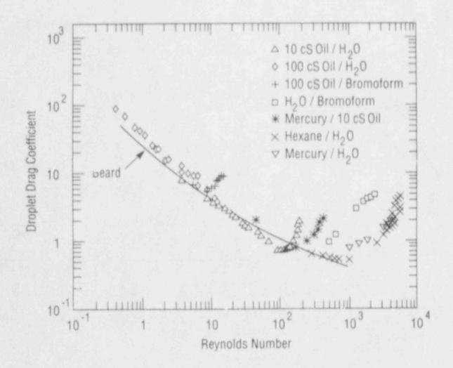
Figure 23. Effect of oscillation and instability on the droplet drag coefficient.
