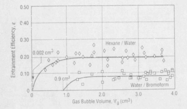
Figure 12. Examples of entrainment efficiencies.
