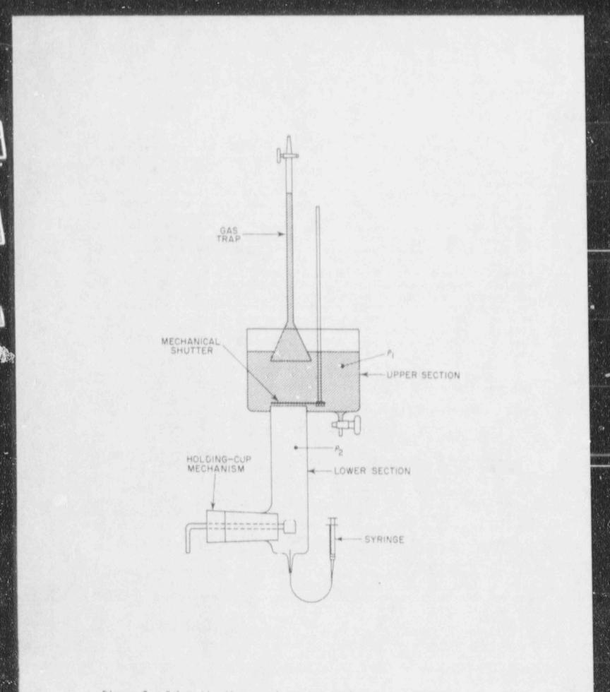
Figure 7. Schematic diagram of experimental entrainment apparatus.
