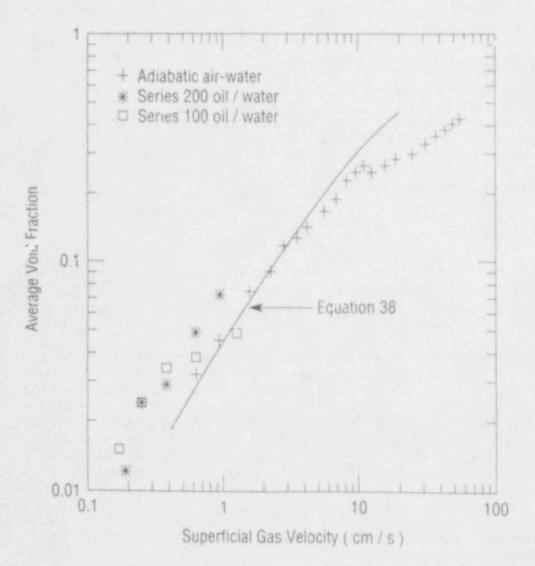
Figure 16. Average void fraction in hubbling pools with bottom gas injection.
