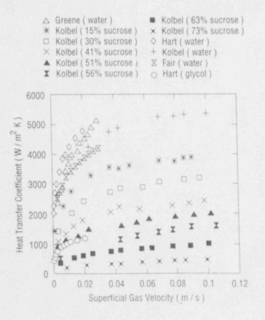
Figure 18. Composite data for bubbling heat transfer coefficients vs. superficial gas velocity: Prandtl number range 2.5-7500.
