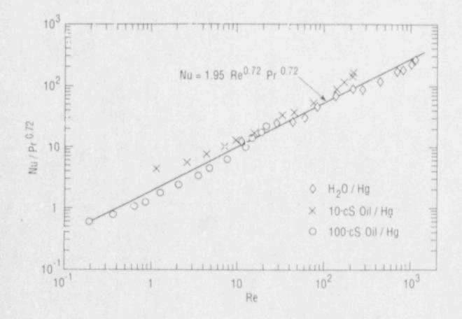
Figure 3. Dimensionless correlation of interfacial heat transfer data.
