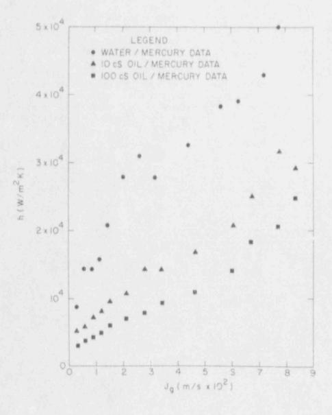
Figure 2. Interfacial heat transfer coefficients vs. superficia! gas velocity.
