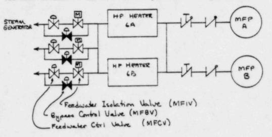
On reactor trip plus safety injection initiation, the main feed control valves and feedwater isolation valves are commanded shut and the main feed pumps are tripped. Continued feedwater flow to a steam generator will occur if both of the valves in the associated feed line fail to close and either main feed pump fails to trip.
