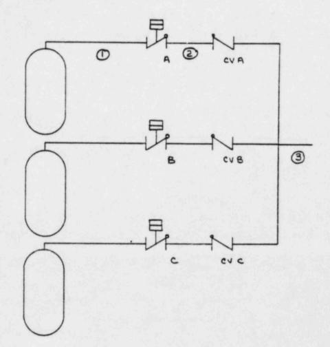
2. Consider potential breaks at location (1) with frequency  $\lambda_1$ , (2) with frequency  $\lambda_2$  and (3) with frequency  $\lambda_3$ . The break locations and valve states for n steam generator blowdown are:
