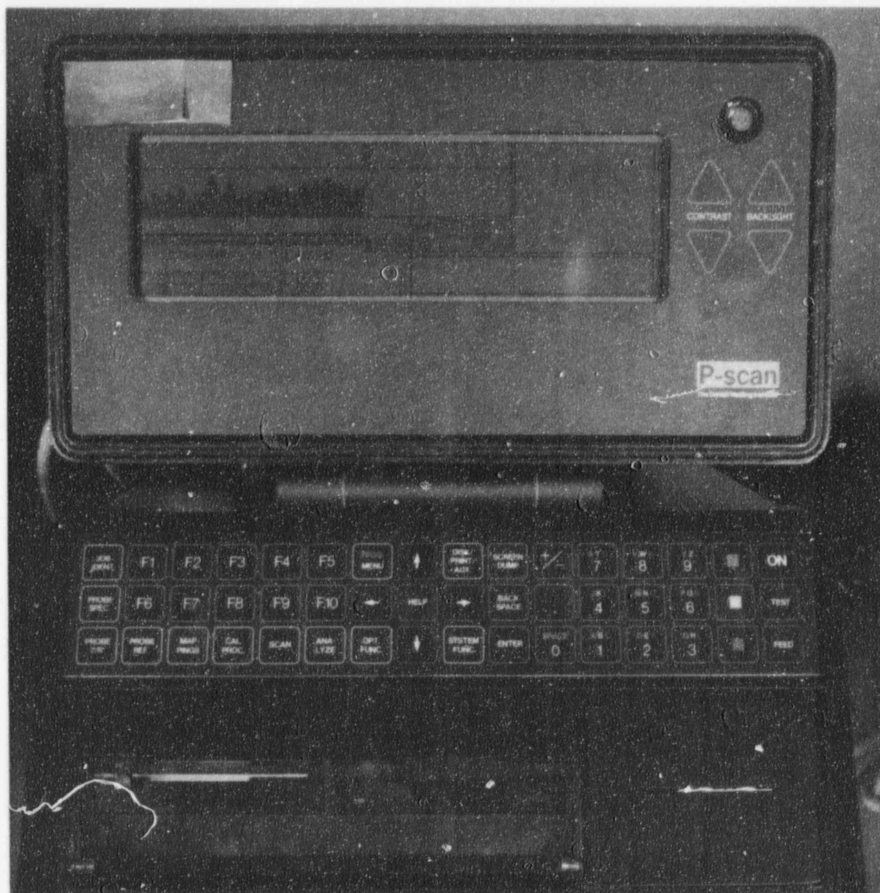
Figure 1.3 PSP-3 system controller and ultrasonic instrument: screen, keyboard, 3-1/2 inch floppy disk drives, 2-1/4 inch strip printer (lower right)
