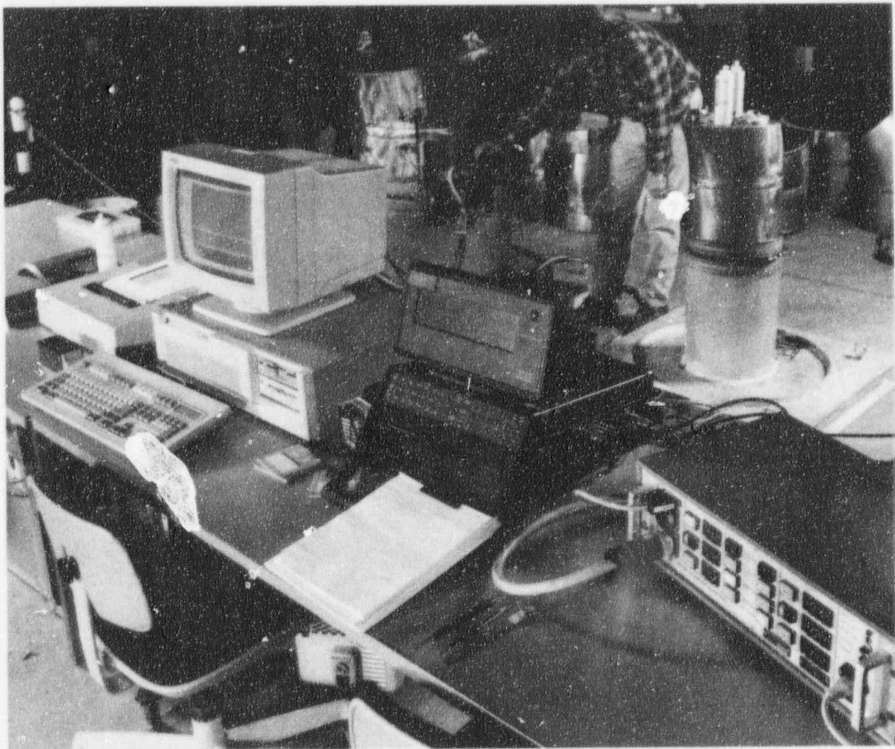
Figure 1.2 P-scan system set up at PNL, showing post-processor (left), PSP-3 (center), scanner control unit (right), and scanner (background)
