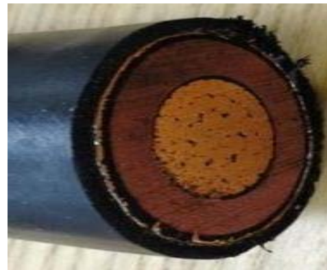
Medium voltage power cable
