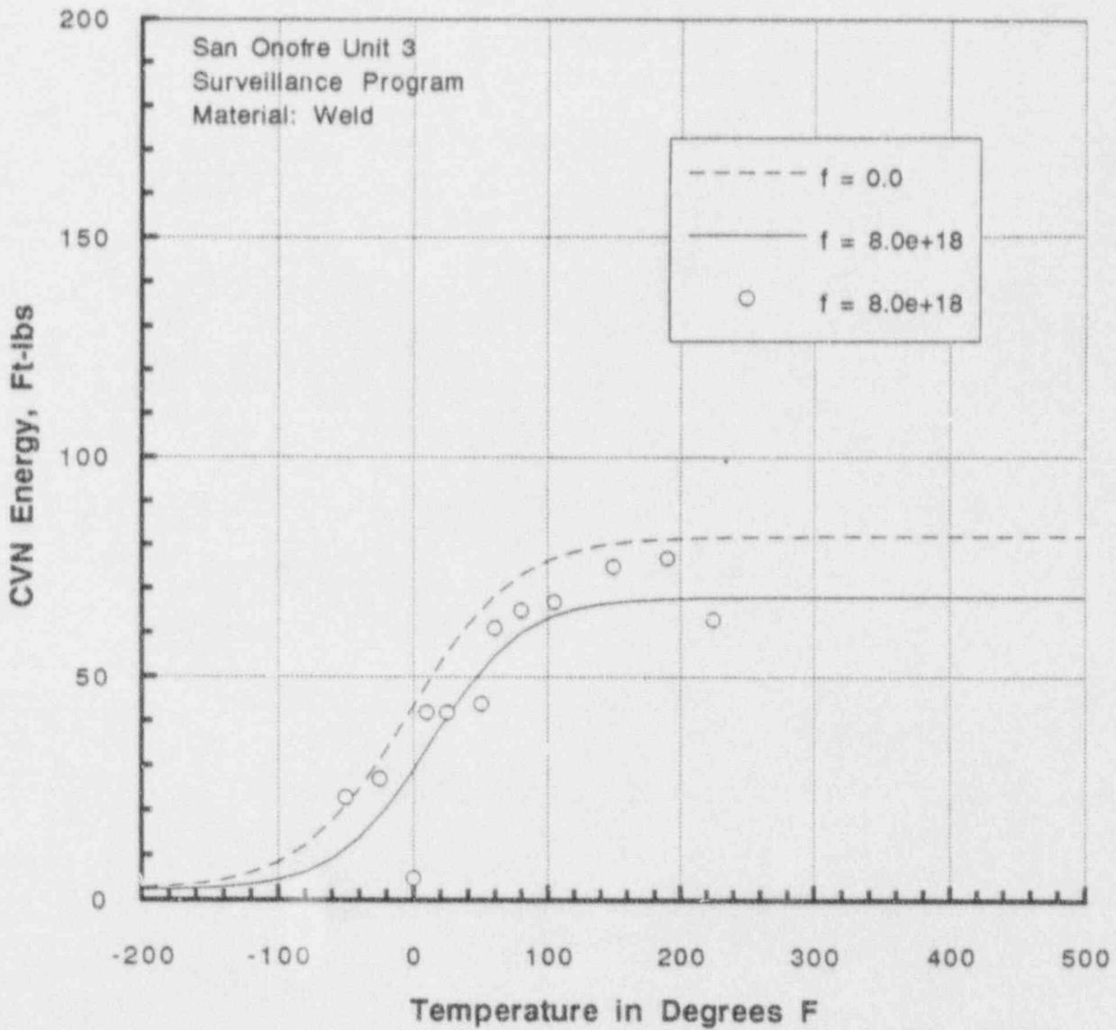
Figure 4-3. SONGS, Unit 3: Comparison of Irradiated  $C_{VN}$  data from Capsule 97 with Unirradiated Baseline Data, Surveillance Weld.
