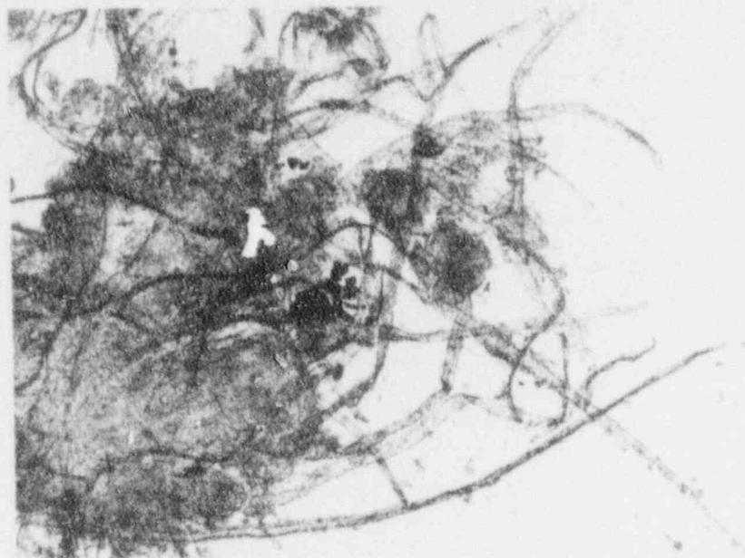
Figure H.6: View of exemplar gasket fibers at 58 X magnification.
