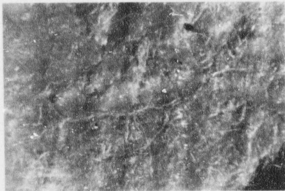
Figure H.5: View of exemplar gasket material at 14 X magnification.
