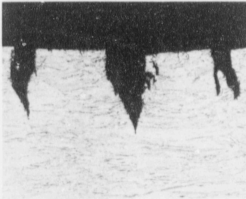
Figure F.4 Photomicrograph Of SSR Specimen Of Alloy CDA 102 Exposed To 0.005M NaNO 2 At 23°C And Polarized To 0.174 Volts (SCE). Specimen Strained To Failure At 1 \times 10^{-6} \text{ sec}^{-1} ; 100X Magnification (Test No. 20).
