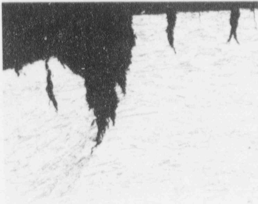
Figure F.5 Photomicrograph Of SSR Specimen Of Alloy CDA 102 Exposed To 1M NaNO 2 At 23°C And Polarized To +0.061 Volts (SCE). Specimen Strained To Failure At 1 \times 10^{-6} \text{ sec}^{-1} ; 100X Magnification (Test No. 17).
