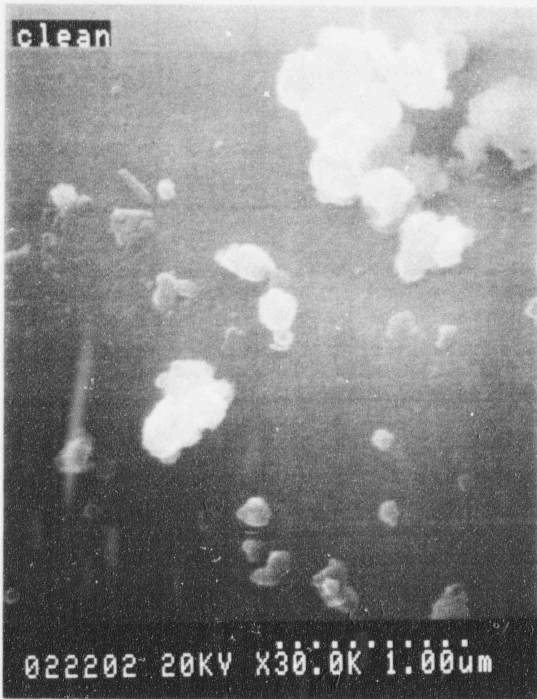
Figure B-22. SEM Photograph of a Clean Fiber Bed (Sample 3-0) at 1 \mu\text{m} Bar Magnification.
