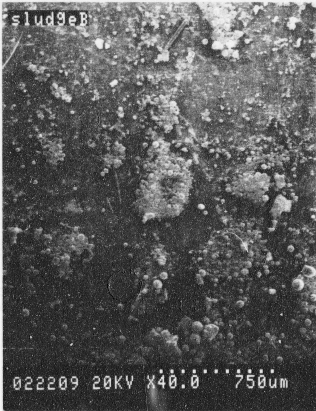
Figure B-15. SEM Photograph of Sludge B as a Dry Powder (Sample 2-0) at 750 \mu\text{m} Bar Magnification.
