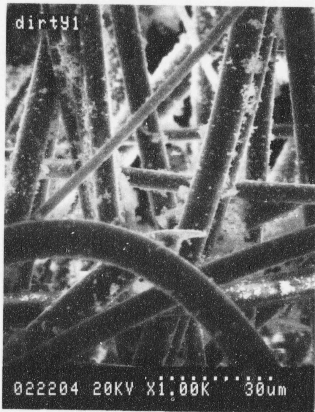
Figure B-24. SEM Photograph of a Lightly Loaded Mixed Bed (Sample 3-1) at 30 \mu\text{m} Bar Magnification.
