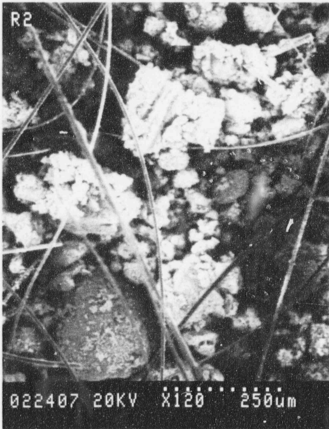
Figure B-27. SEM Photograph of a Heavily Loaded Mixed Bed (Sample 3-2) at 250 \mu\text{m} Bar Magnification.
