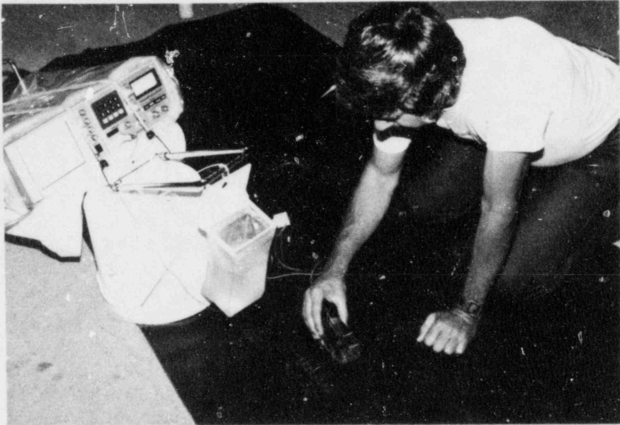
Figure 15. Ultrasonic impedance plane instrument being used for seam inspection
