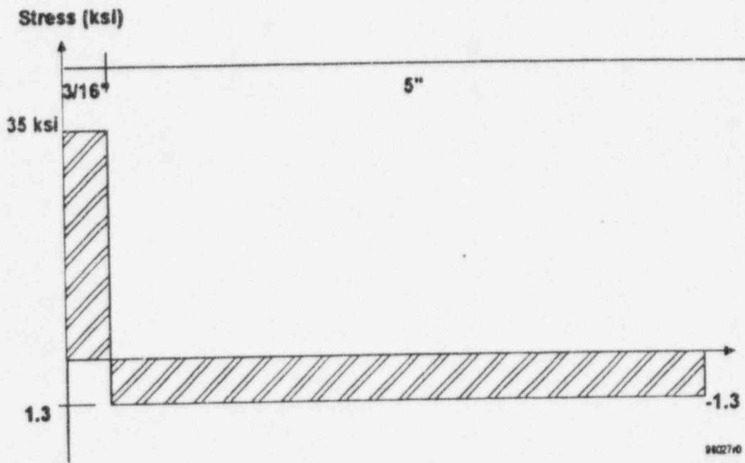
Figure 3. Clad Residual Stress
