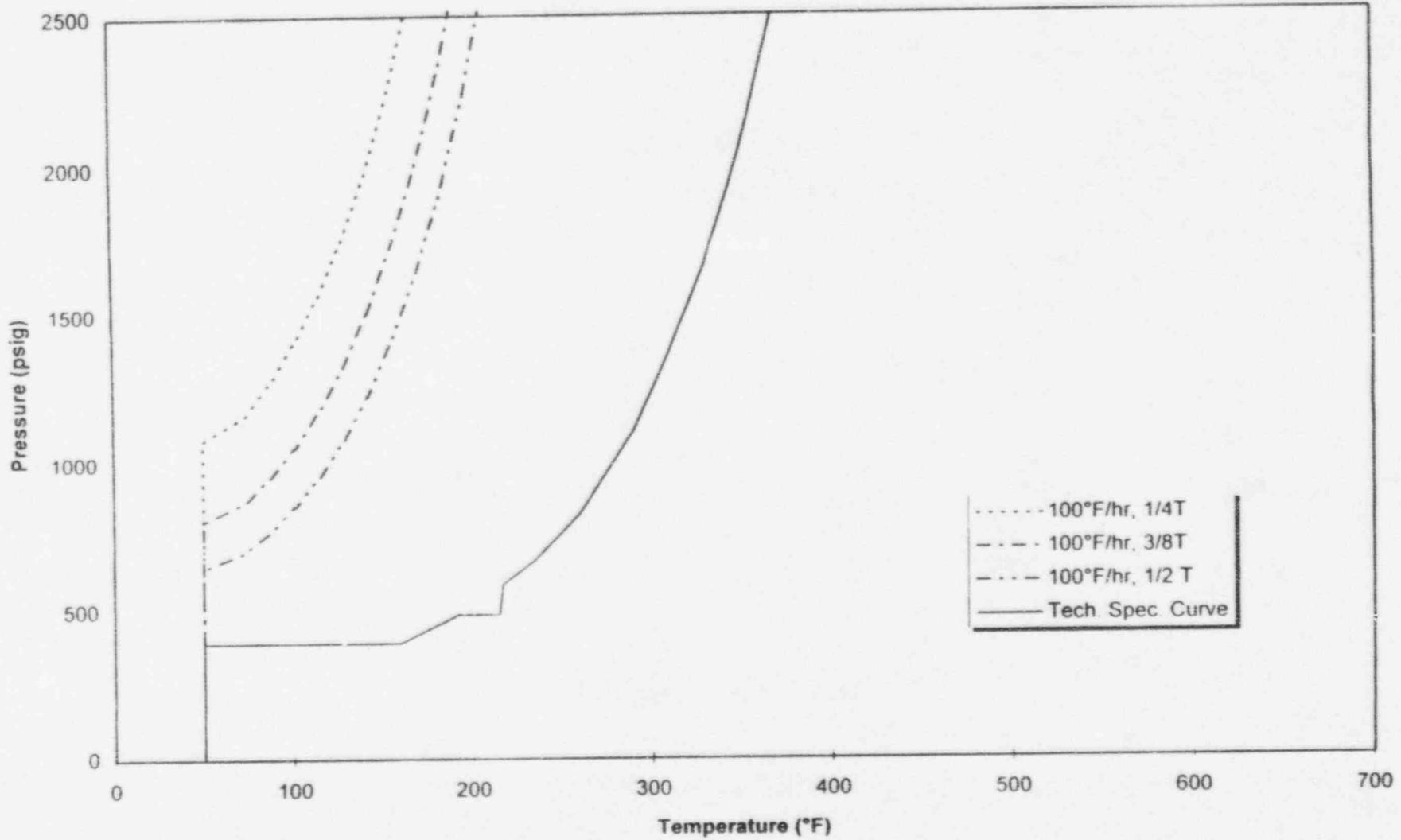
Figure 4. P-T Curve for Bottom Head Region for Flaw Sizes of 1/4T, 3/8T and 1/2T
