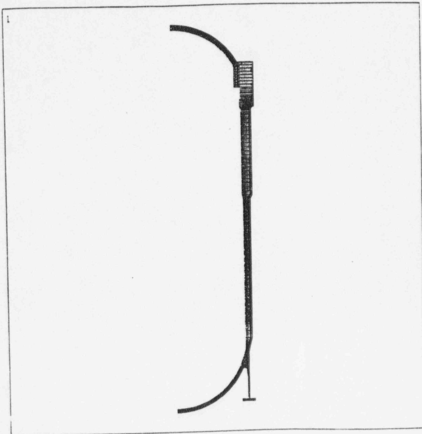
Figure 2. Reactor Vessel Axisymmetric Finite Element Model
