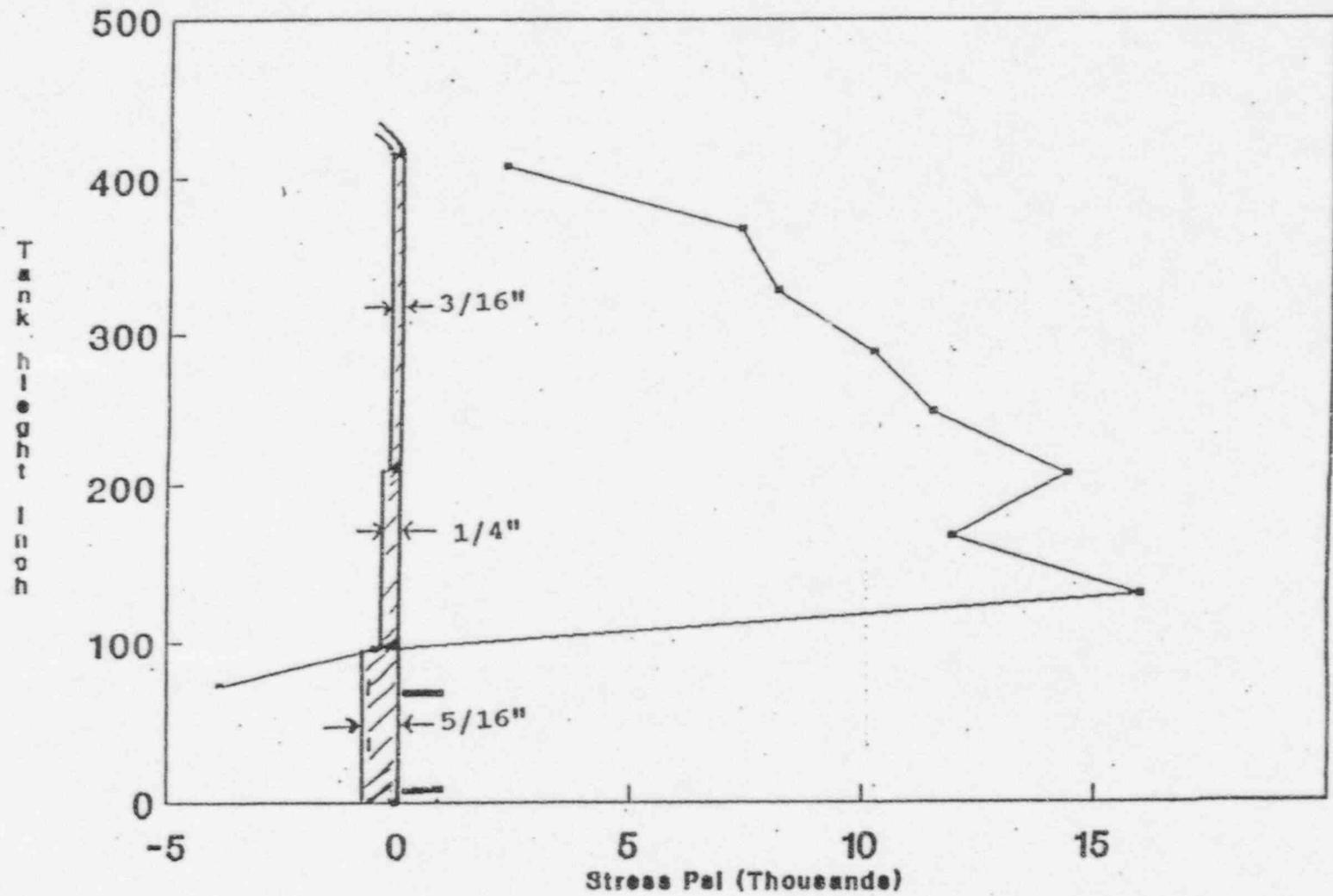
Figure 5.8 Hoop Stress Distribution in the Tank Shell
