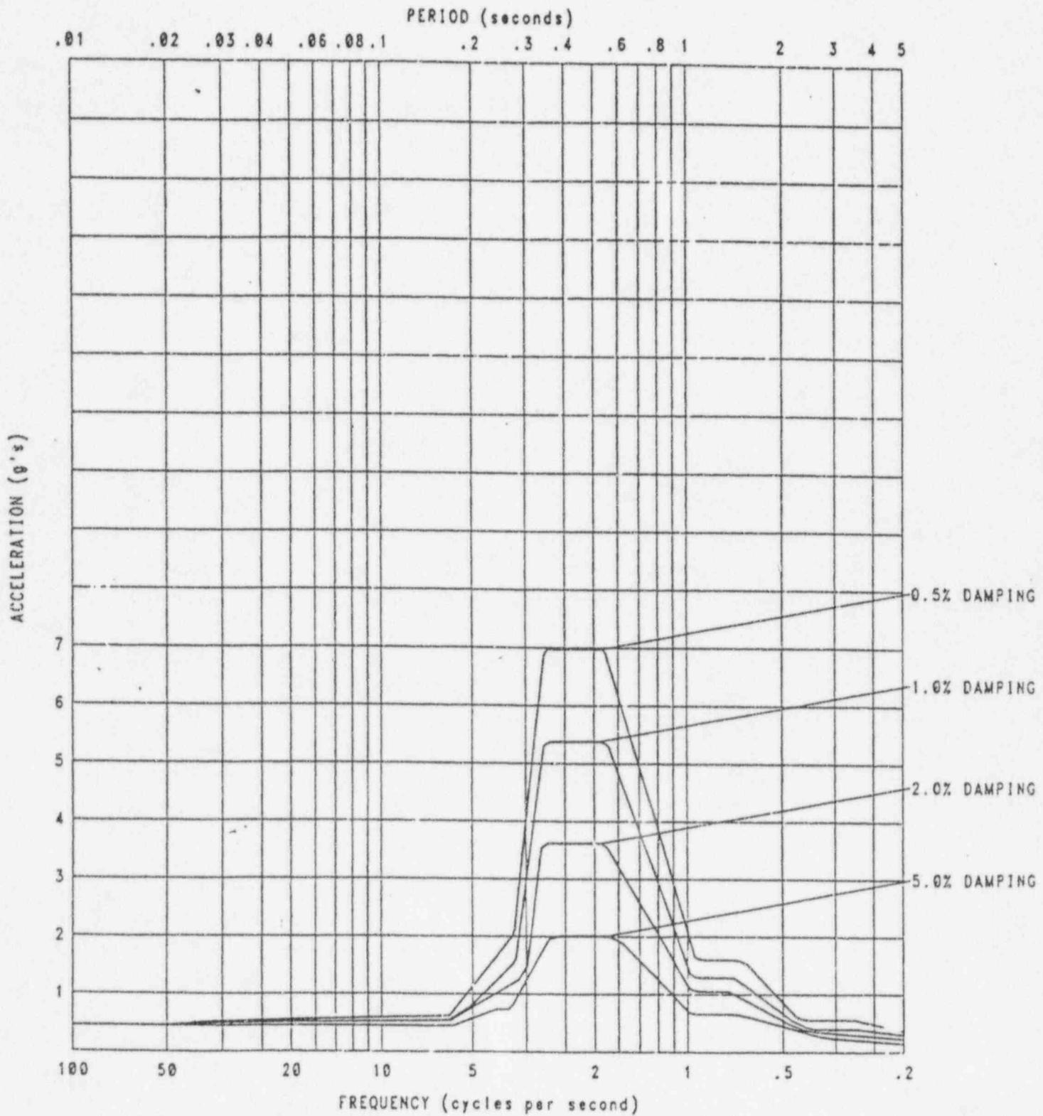
Operating Basis Earthquake Vertical Acceleration Response Spectra, Elevation 9'-0" of Auxiliary Building
