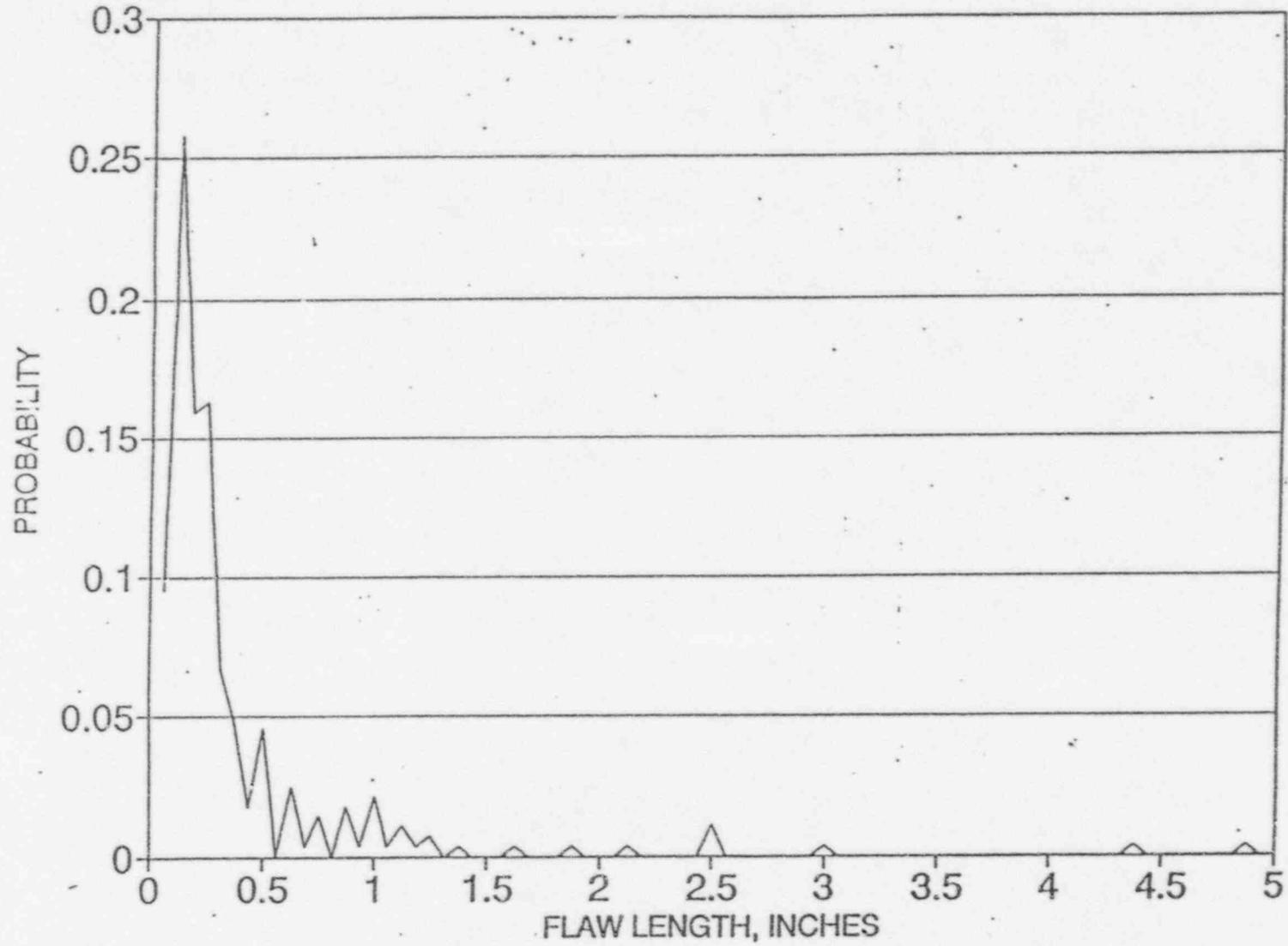
Figure 5.5 Weld Defect Size Population Distribution for Unit-2 PPMS Tank (T056)
