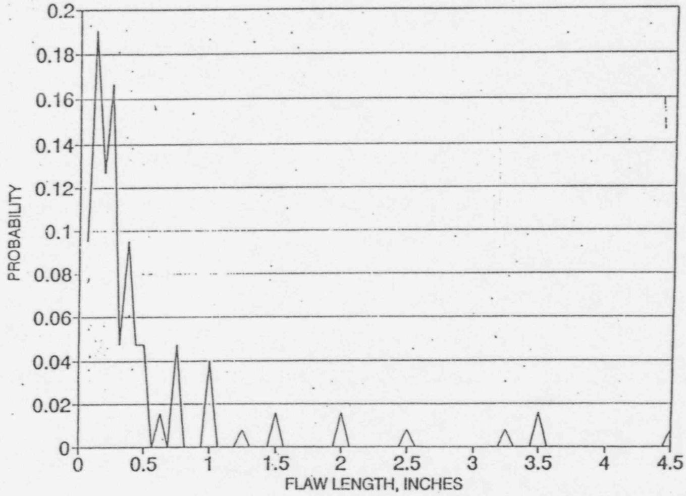
Figure 5.7 Weld Defect Size Population Distribution for Unit-3 PPMS Tank (T055)
