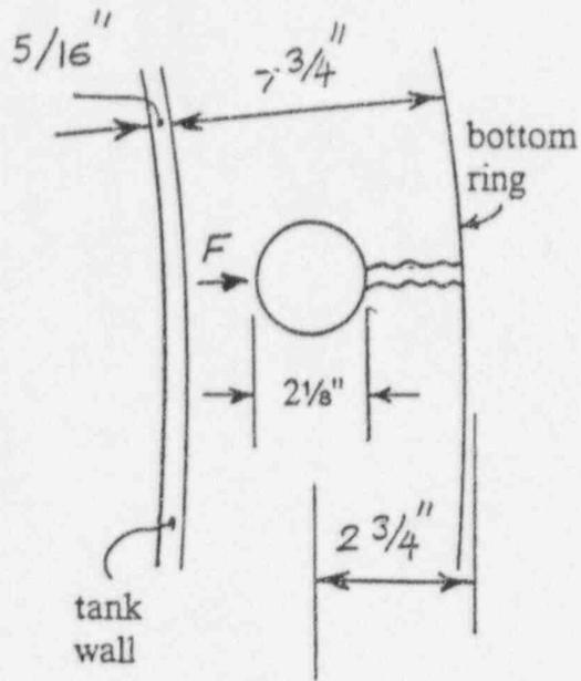
(a) Tearout Failure
