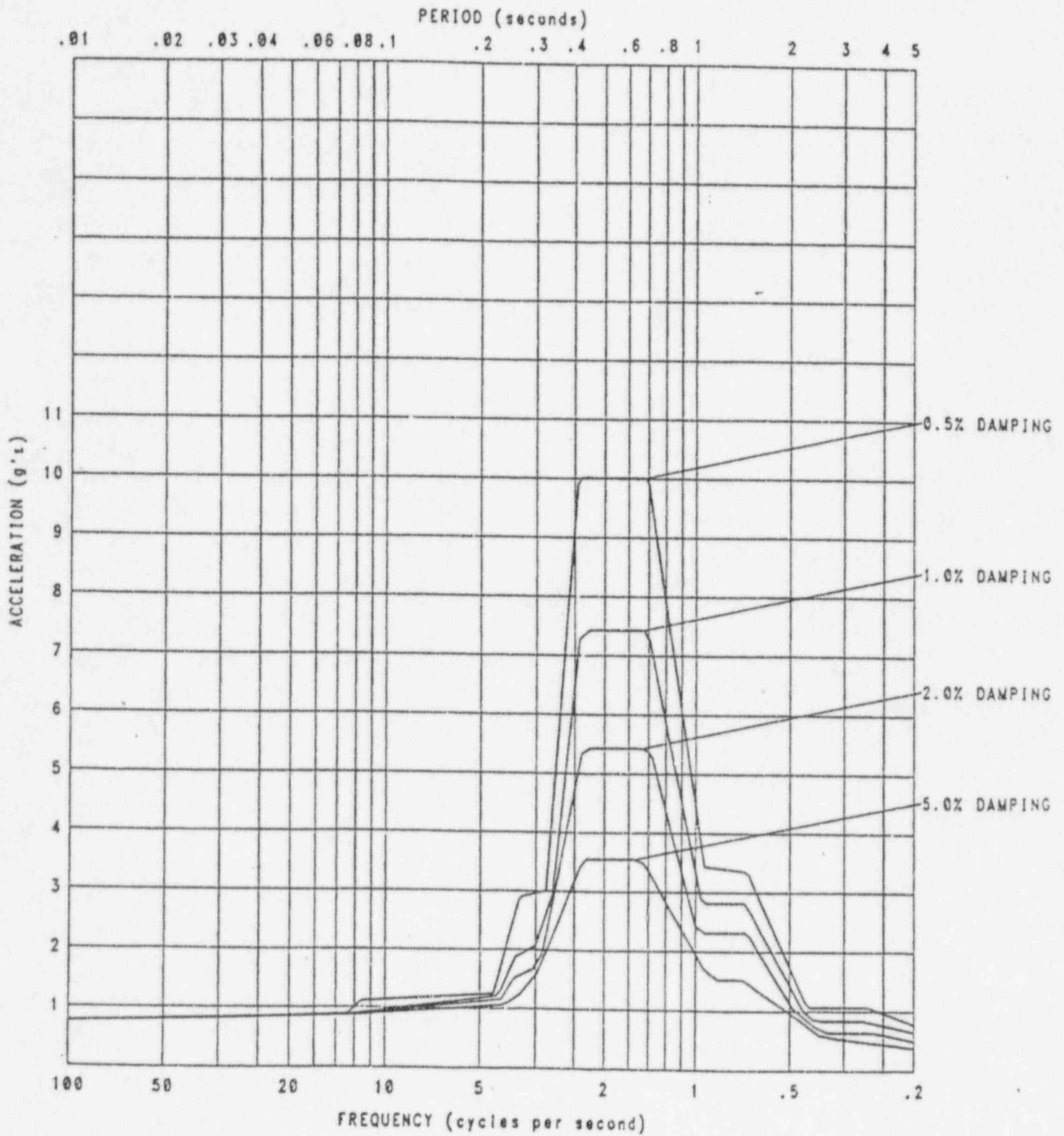
Design Basis Earthquake Vertical Acceleration Response Spectra, Elevation 9'-0" of Auxiliary Building
