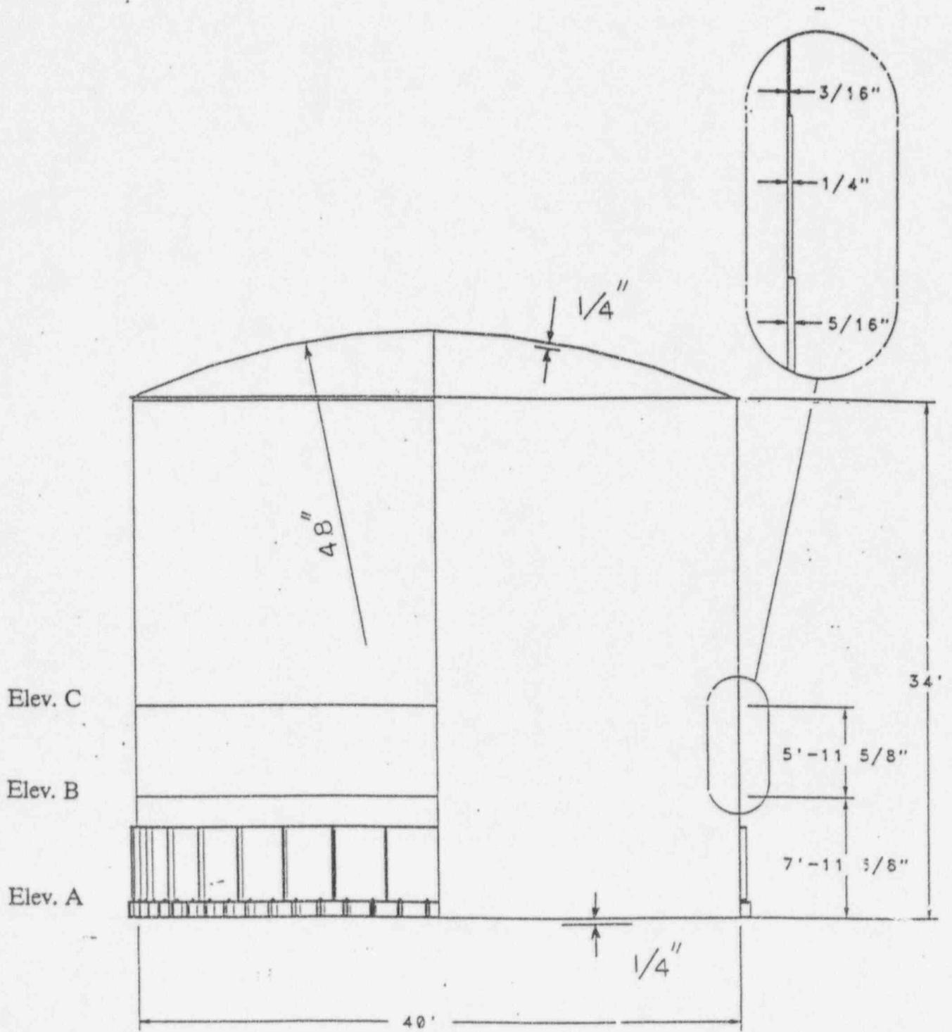
Figure 4.1 Main Dimensions of the PPMS tank
