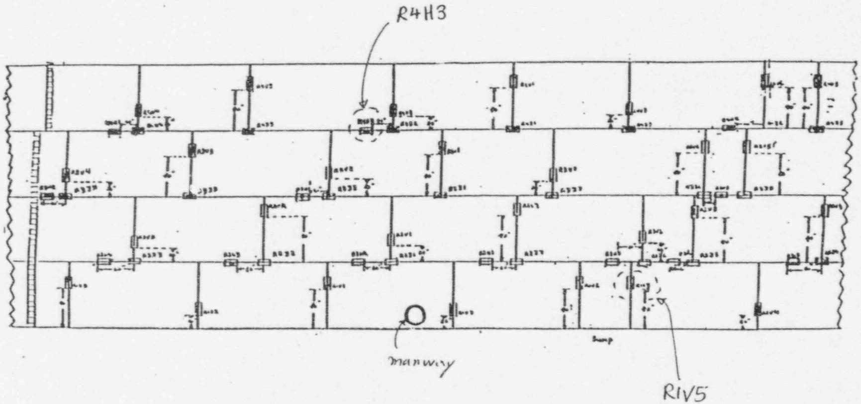
Figure 2 Unit-3 PPMS Tank Radiographic Examination Map
