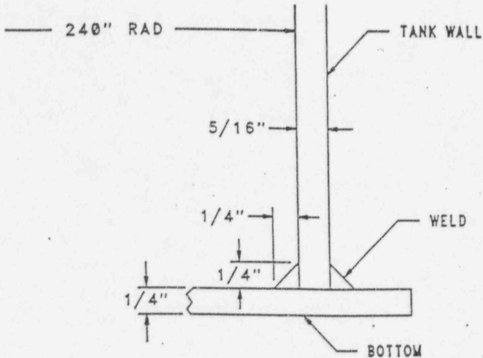
The tank shell is welded to the bottom by a double 1/4" fillet weld in accordance with API-650, Section 3, while ND-4746.2 calls for a full penetration weld. To address this deviation, the weld was evaluated for both shear and moment loads using ND-3852.6 shear allowable. The analysis results show that the existing fillet weld meets the ASME Code allowable stresses under DBE loading.
