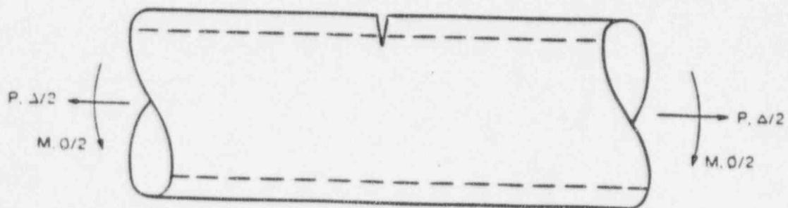
6.2 Circumferential Crack Leak Rate Calculations:
