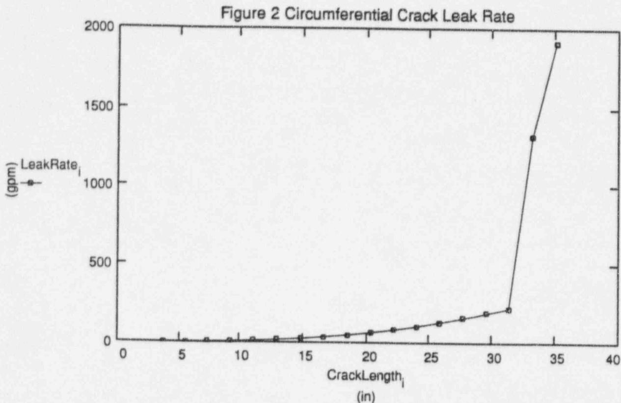
The leak rate prior to a crack length of approximately 32" is choked. Once the flaw length reaches this limit and the flow through the crack is no longer choked, the leak rate increases significantly.
