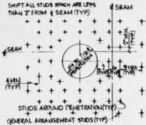
TYPICAL SPACING DET FOR 10"  $\phi$  TO 1.6"  $\phi$  PENETRATIONS
