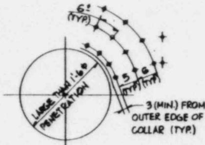
TYPICAL SPACING DETAILS FOR LARGER THAN 1.6"  $\phi$  PENETRATIONS (UNLESS NOTED)
