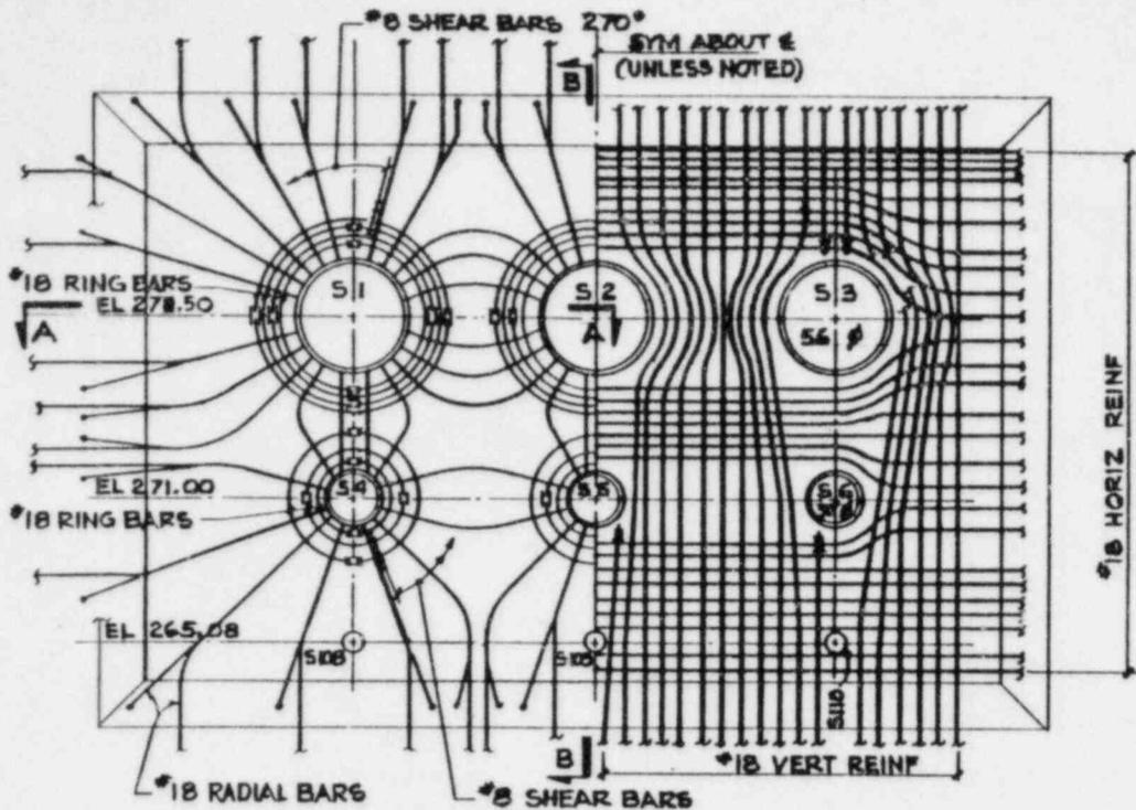
DEVELOPED ELEVATION AT M.S., F.W. & A.F.W. SLEEVES
