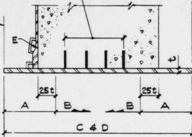
A - DIV. BOUNDARY FOR ASME CODE, SECT III, DIV 1 WITH SUBSECTION CA (FOR NEW MATERIAL & SERVICES FURNISHED AFTER 4-29-1977) FOR TYPE II & III PENETRATION SLEEVES.
