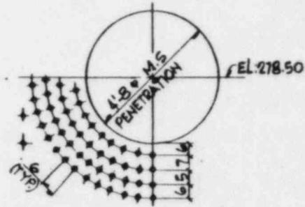
TYPICAL SPACING DETAIL FOR 4.8"  $\phi$  M.S. PENETRATIONS
