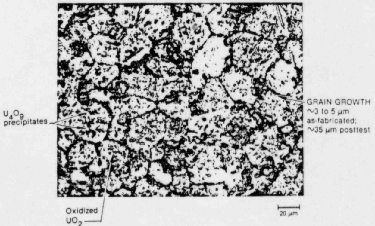
Figure 6. Postirradiation Microstructure of the SFD-ST Fuel Remains, Indicating Grain Growth to 35 microns and UO_2 Oxidation to U_4O_9 -Inclusions.
