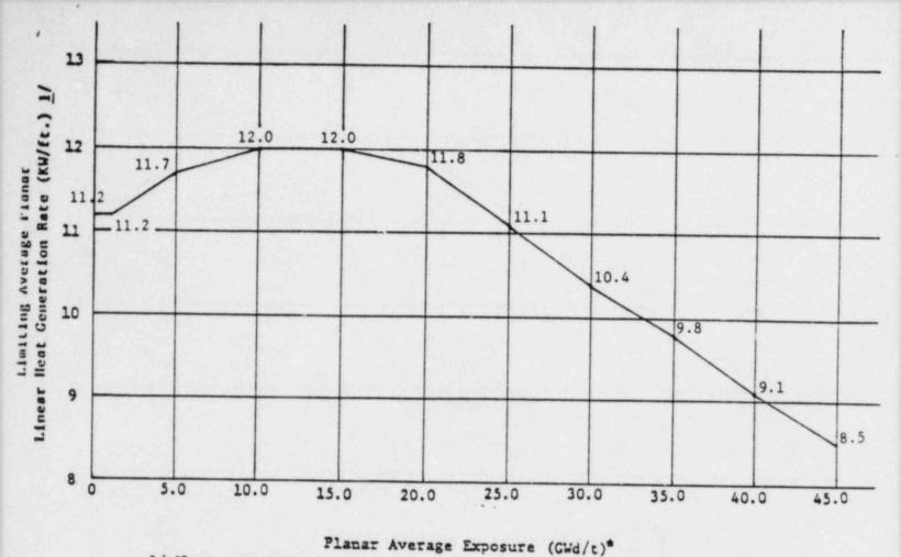
1/ When core flow is equal to or less than 70% of rated, the MAPLEGR shall not exceed 95% of the limiting values shown.
