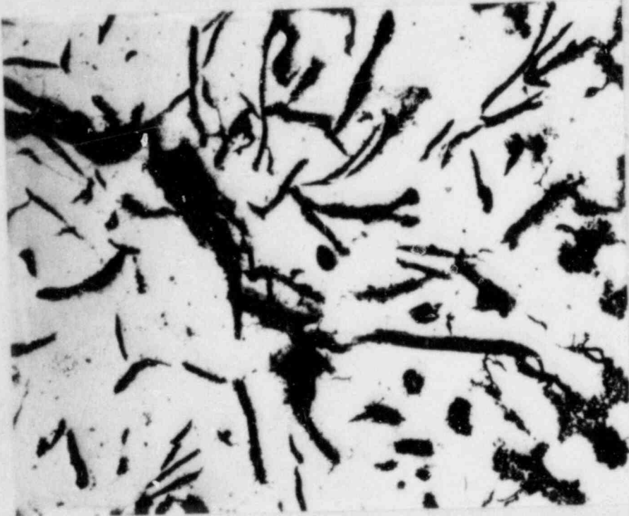
Tip of Casting Shrinkage Crack
