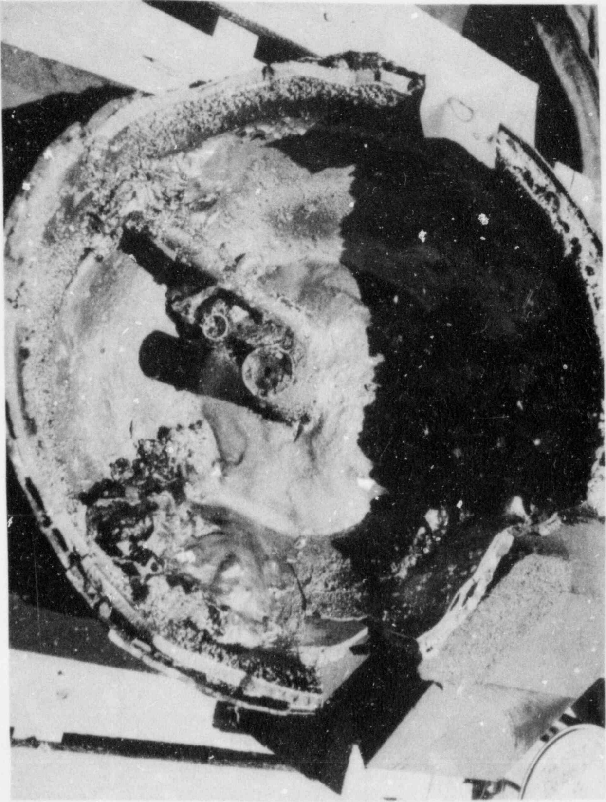
Figure V.7 Bottom of Melt Crucible with Melt Charge Removed
