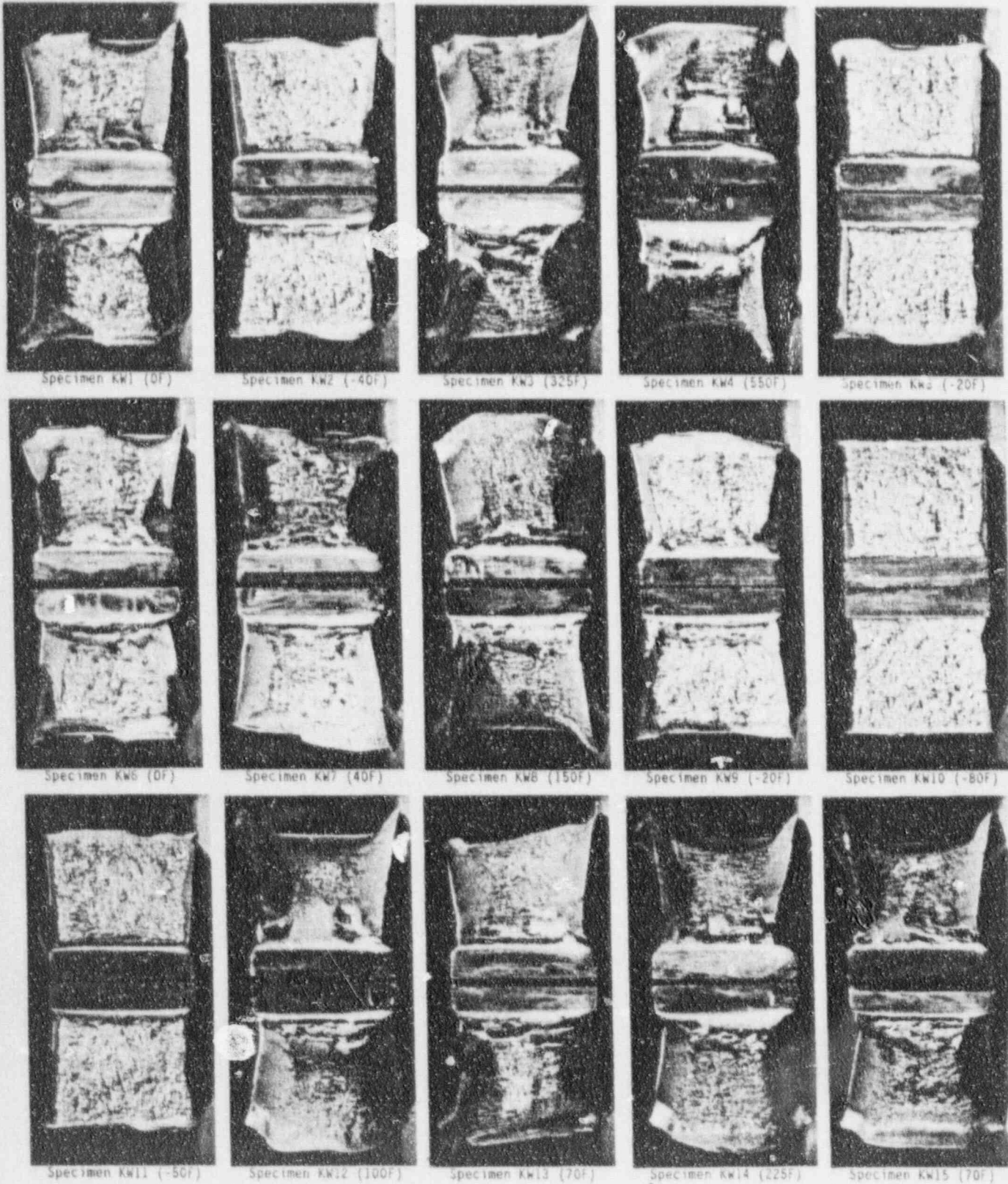
Figure 3-20. Photographs of Charpy Impact Specimen Fracture Surfaces - Weld Metal
