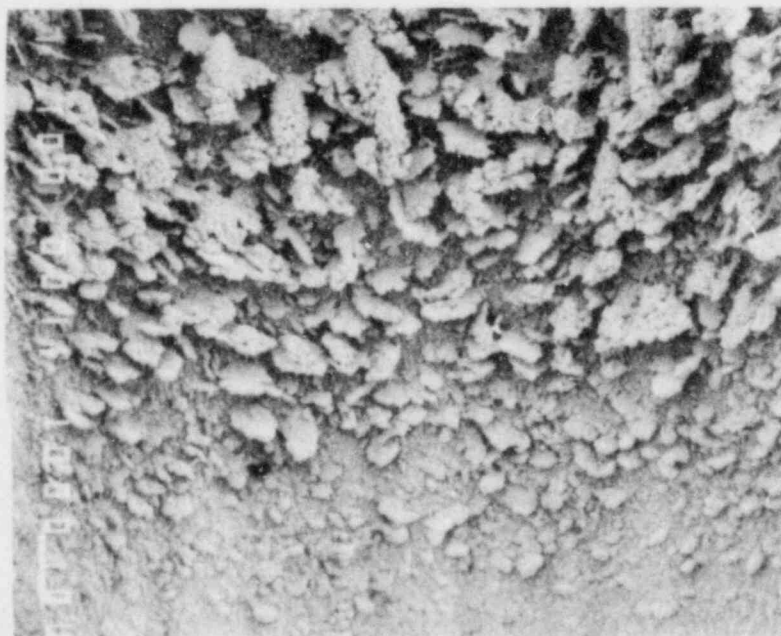
Figure 1.1.3 SiC Formed in Section 11 in Figure 1.1.1. Magn. 10X.
