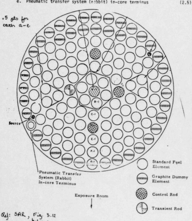
$K_{\circ}8$  How does the fuel element worth (compared to water) change as you move from core ring G to F to E to D to C to B?
