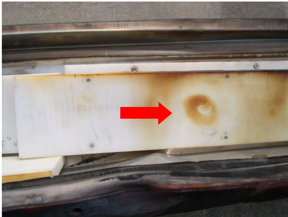
Figure 3-44 Localized Melt Spot in Lid Moderator Block
