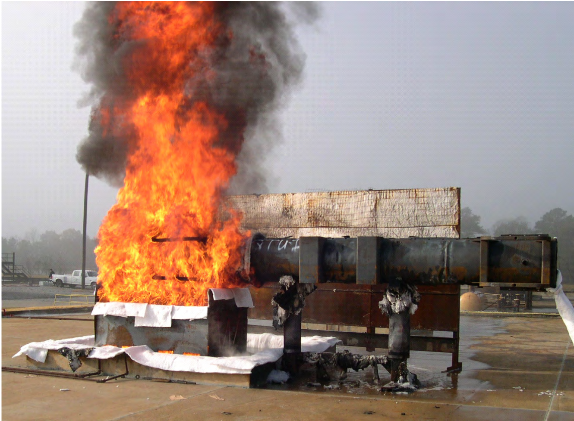
Figure 3-19 December 15, Impact Limiter Burn Test
