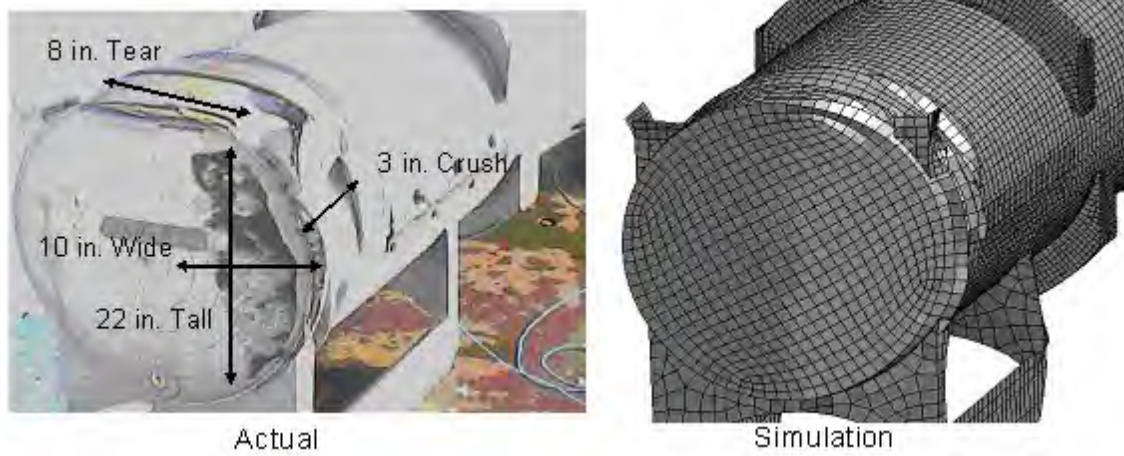
Figure 2-84 Outerpack Deformations at Bottom Nozzle End of Package
