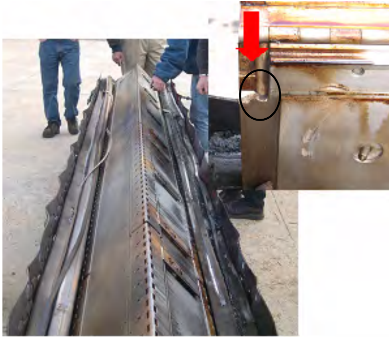
Figure 2-149 CTU Clamshell After Drop and Fire Tests
