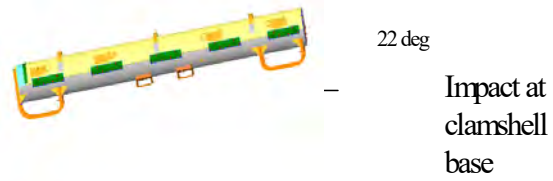
Figure 2-135 QTU Test Series 2 Drop Orientations
