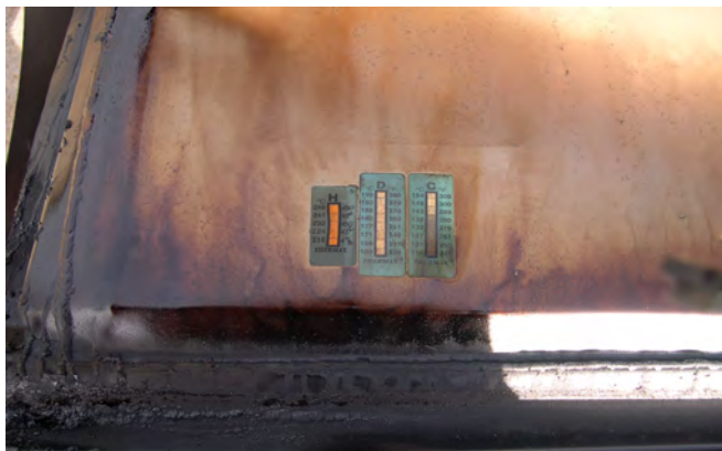
Figure 3-46 Temperature Strip Set After Fire Test
