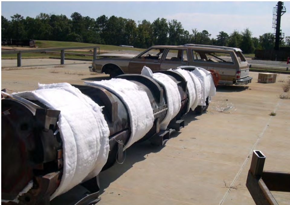
Figure 3-11 Package Exterior Wrapped with Ceramic Fiber Insulation
