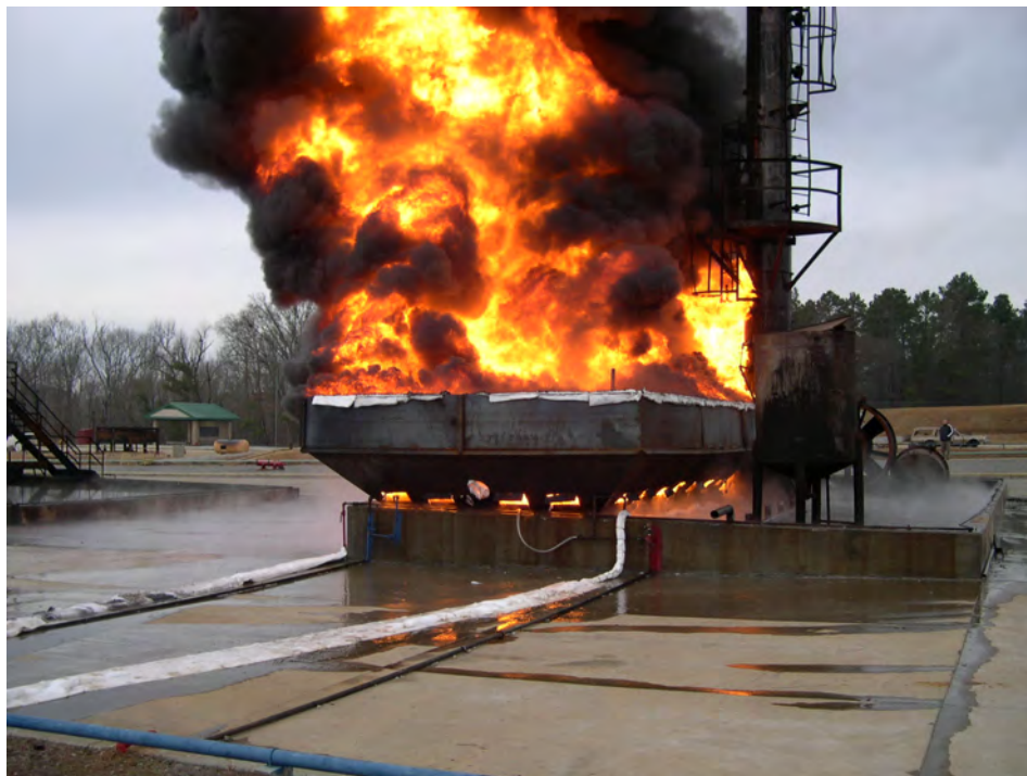
Figure 3-4 December 15, Impact Limiter Burn Test
