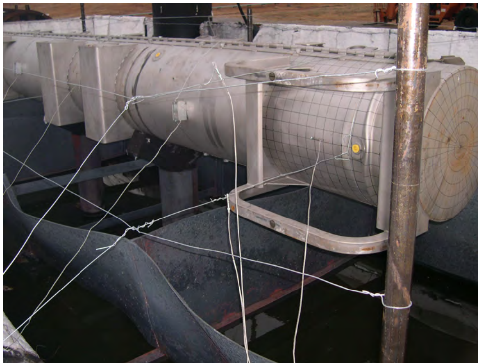
Figure 3-32 Test Stand for Fire Test
