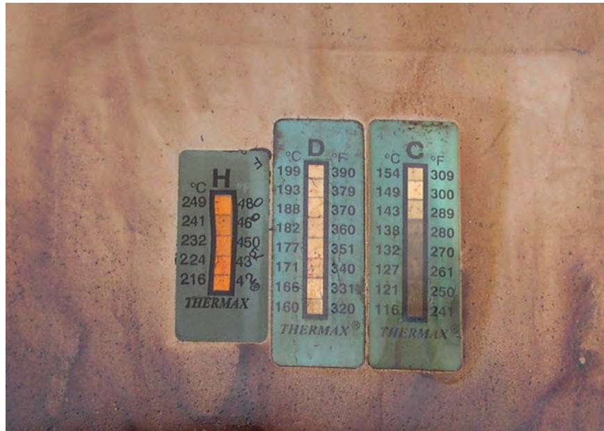
Figure 3-8 Temperature Strip Condition After CTU Burn Test
