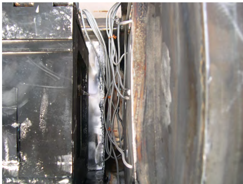
Figure 3-23 Outerpack Internals after December 15 Burn Test
