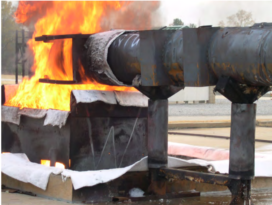
Figure 3-25 December 16 Impact Limiter Burn
