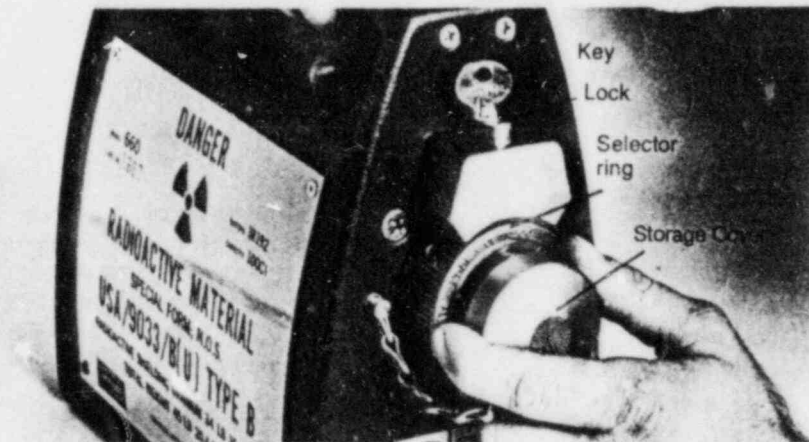
FIGURE 2.4 - Unlock the exposure device with the key provided and turn the selector ring from the LOCK position to the CONNECT position. When the ring is in the CONNECT position, the storage cover will disengage from the exposure device as shown.
