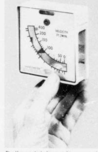
The Vaneometer's large scales are easy to read. Both sides have factory calibrated scales. Recessed bubble level at top helps insure accurate readings.
