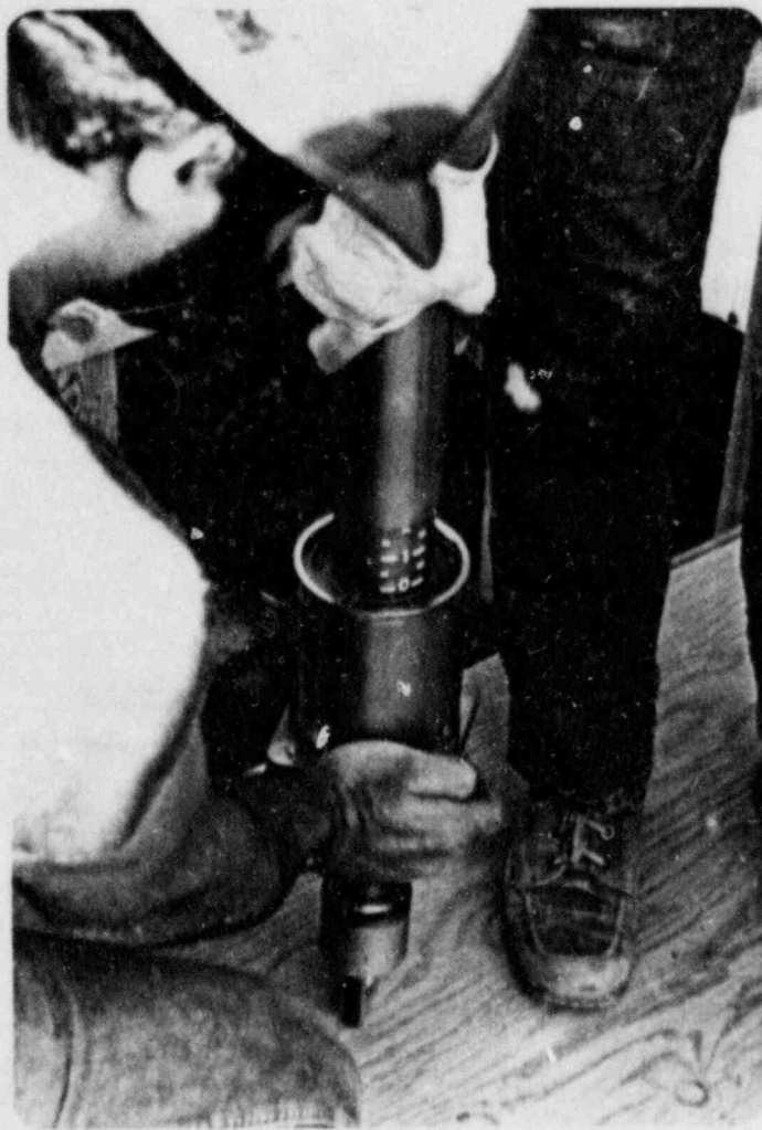
Photograph 3.1.1 Stroking of a mechanical shock suppressor.
