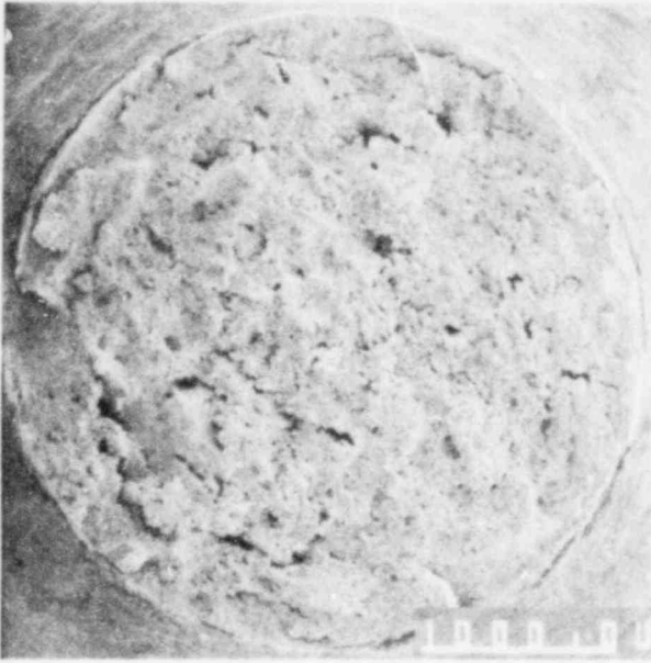
Figure 95. 27X SEM Photo of Fracture Face for Specimen #41.
