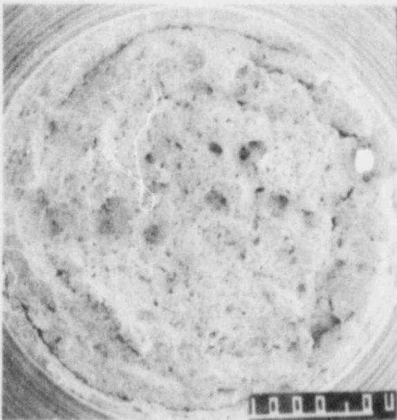
Figure 69. 27X SEM Photo of Fracture Face for Specimen #28.
