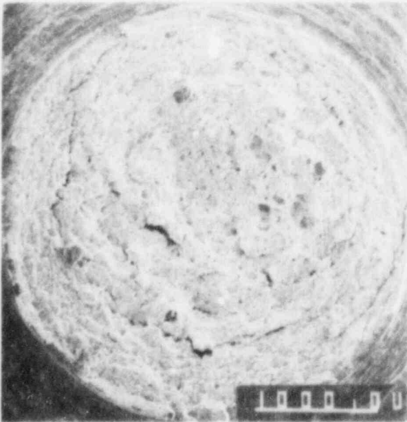
Figure 17. 27X SEM Photo of Fracture Face for Specimen #2.
