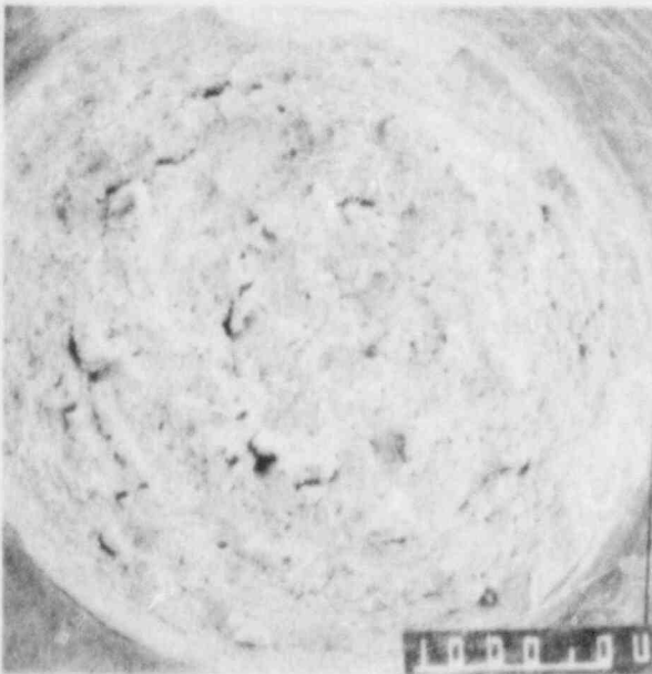
Figure 37. 27X SEM Photo of Fracture Face for Specimen #12.
