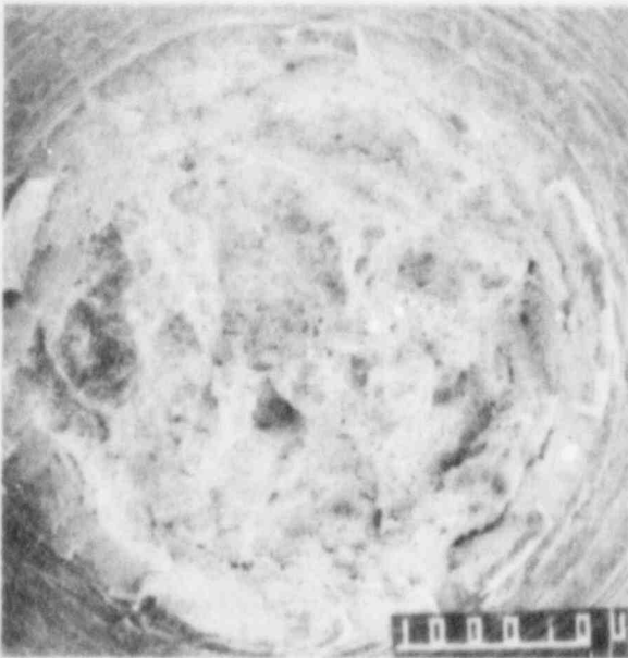
Figure 73. 27X SEM Photo of Fracture Face for Specimen #30.
