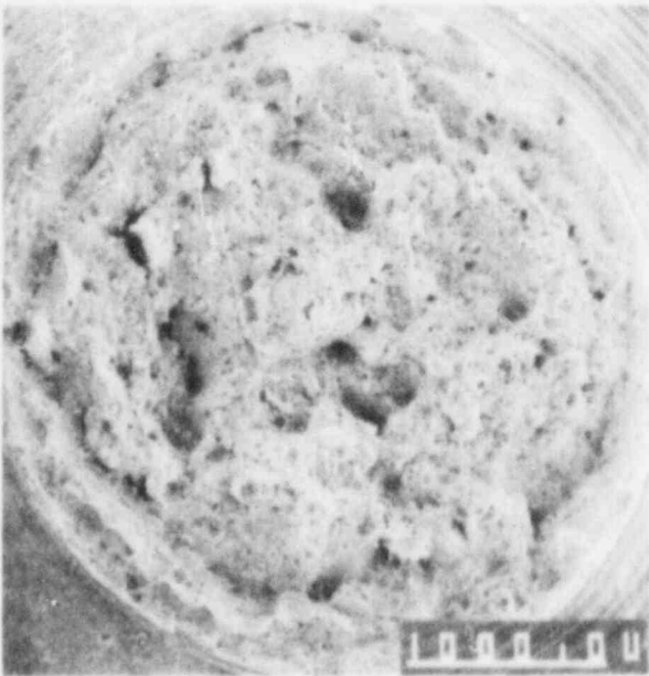
Figure 49. 27X SEM Photo of Fracture Face for Specimen #18.
