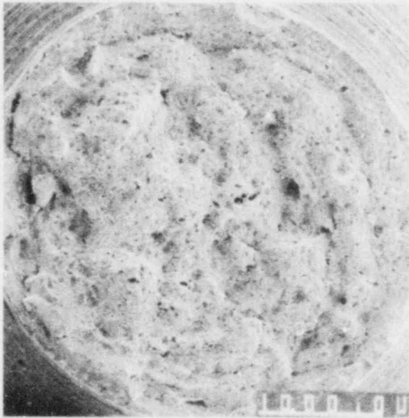
Figure 125. 27X SEM Photo of Fracture Face for Specimen #56.
