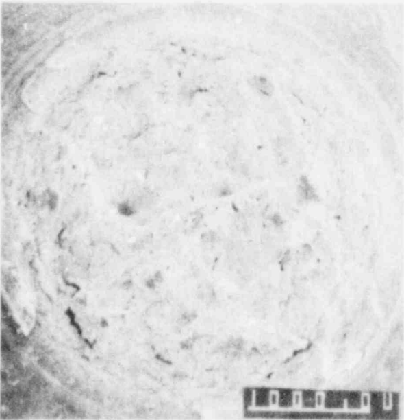
Figure 25. 27X SEM Photo of Fracture Face for Specimen #6.
