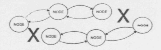
WHEN THE LOOP IS BROKEN OR WIRE TO WIRE SHORT AT TWO DIFFERENT LOCATIONS, EACH SECTION WILL COMMUNICATE TO THE NODES CONNECTED PROVIDING TWO DEGRADED LOOPS.
