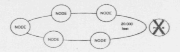
SYSTEM CAN STILL OPERATE WITH A FAILED NODE.
