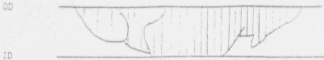
Sketch of Burst Crack
