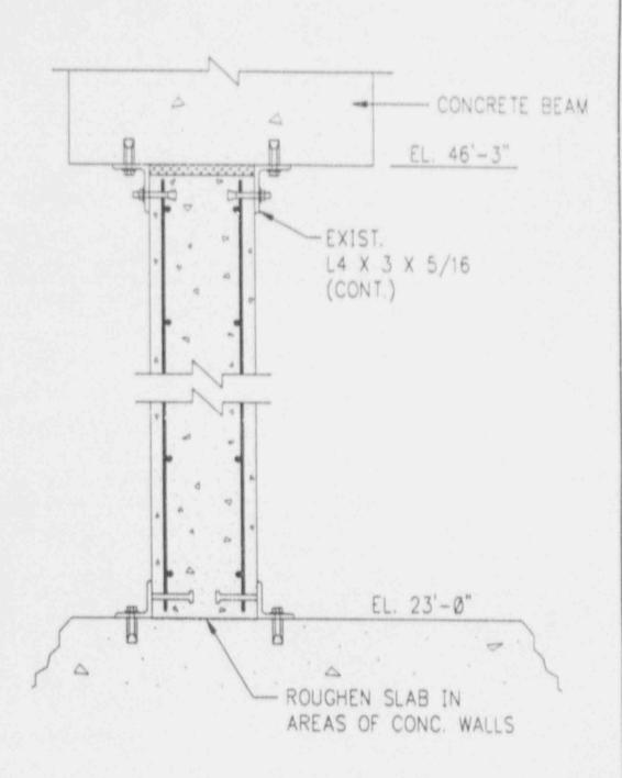
REINFORCED CONCRETE PANEL (AS DESIGNED)
