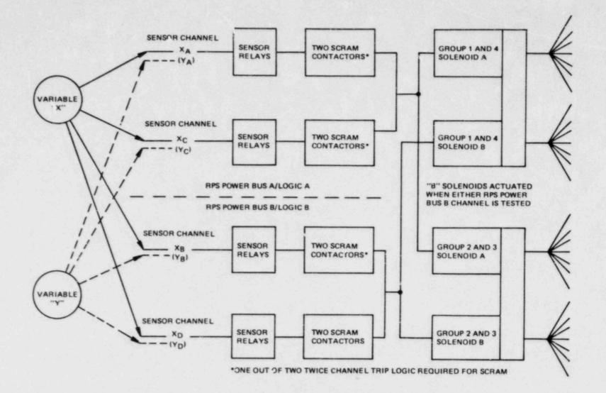
Figure 1. RPS Relay Logic Configuration
