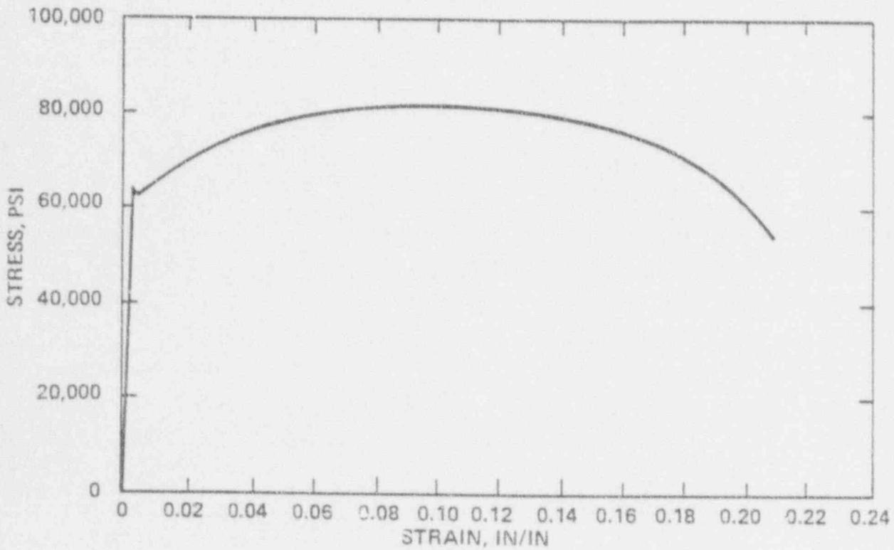
Figure VI-2: Stress-Strain Record of Tensile Test
