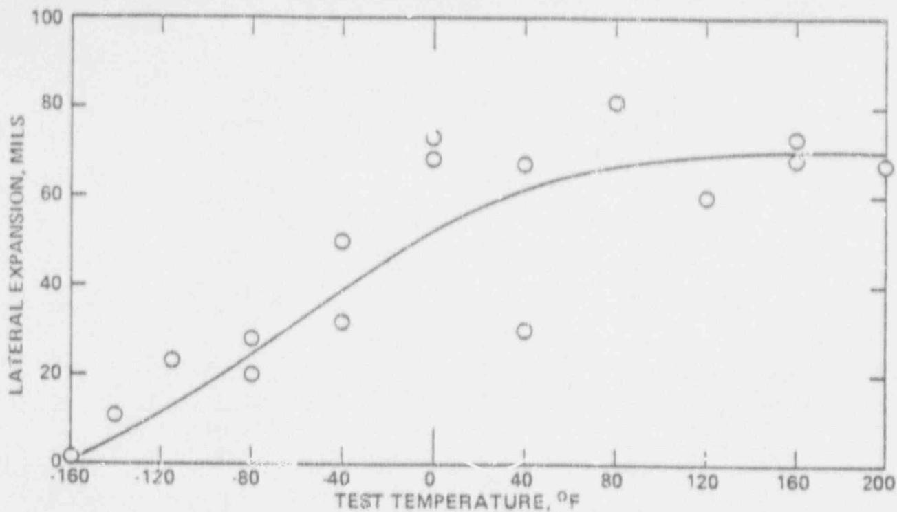
Figure VI-15: LATERAL EXPANSION vs TEMPERATURE
