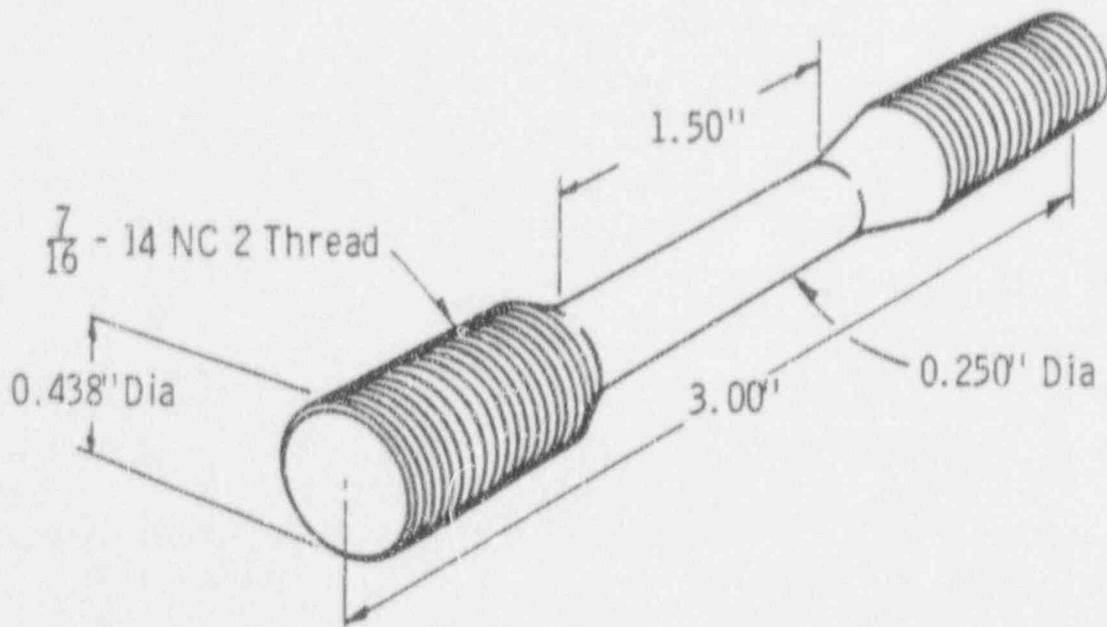
FIGURE: 8-2. Typical Tensile Specimen
