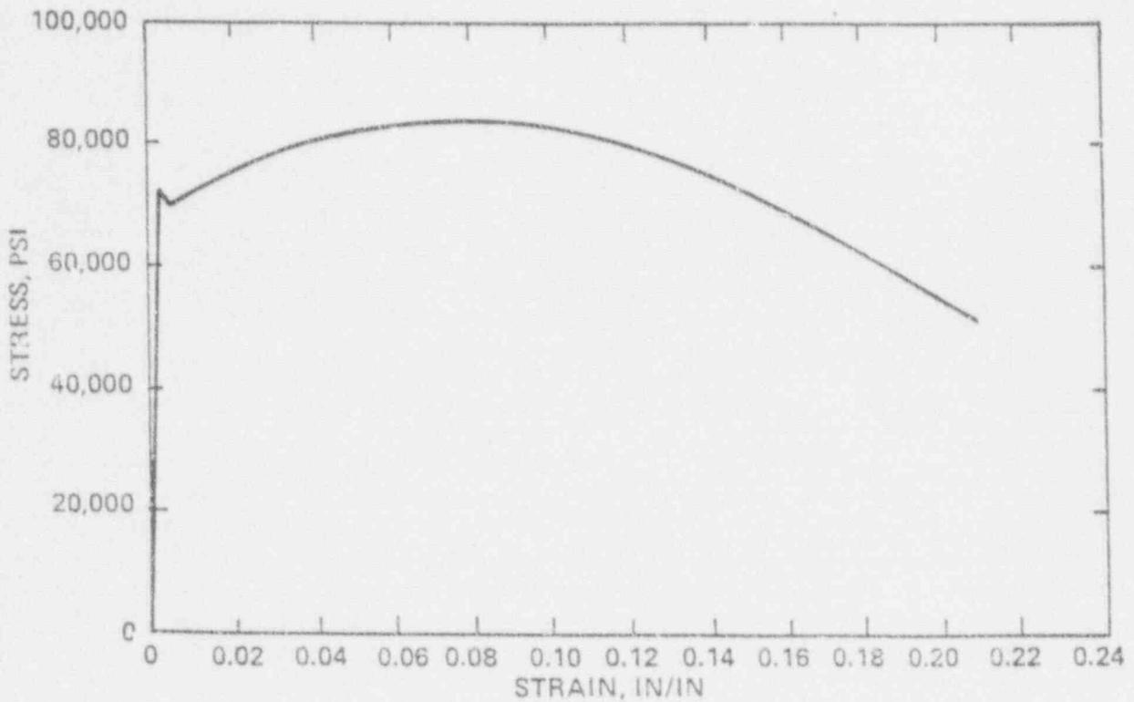
Figure VI-8: Stress-Strain Record of Tensile Test
