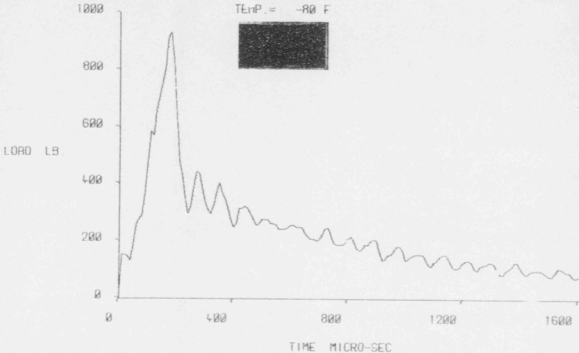
Figure VIII-1:  $PIC_y$  Load Record for Base Metal Plate D-4802-2 (WR)
