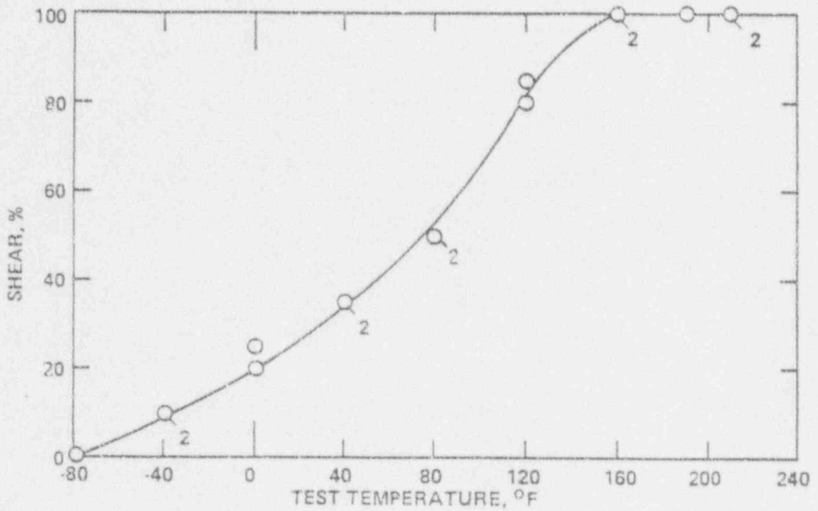
Figure VII-8: SHEAR vs TEMPERATURE
