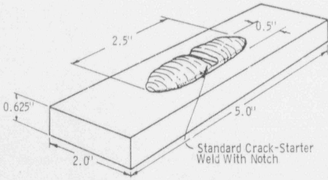
FIGURE: A-2. Typical Drop Weight Specimen
