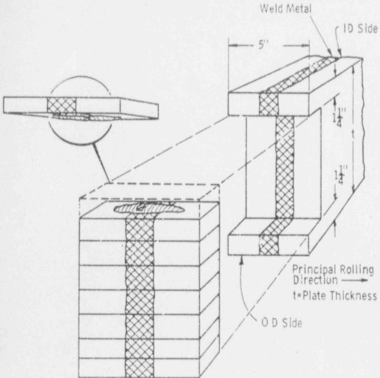
FIGURE: A-4. Location of Drop Weight Specimens Within Weld Metal Test Material
