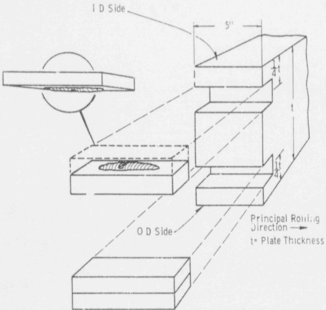
FIGURE: A-3. Location of Drop Weight Specimens Within Base Metal Test Material
