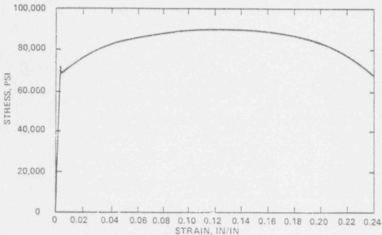
Figure VI-4: Stress-Strain Record of Tensile Test
