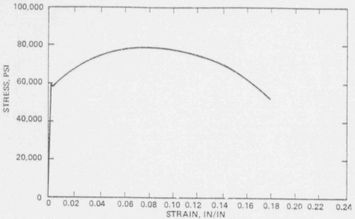
Figure VI-11: Stress-Strain Record of Tensile Test
