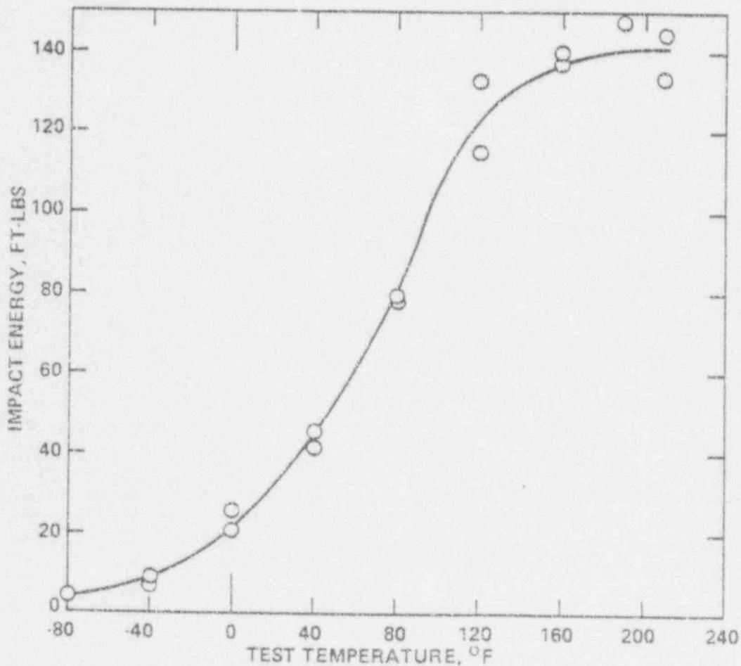
Figure VII-6: IMPACT ENERGY vs TEMPERATURE
