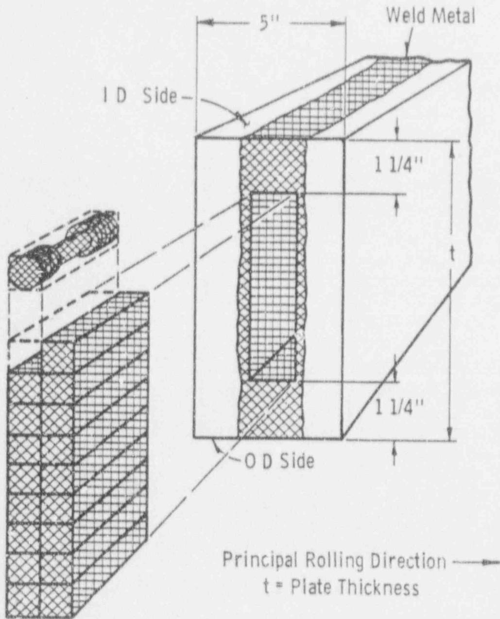
FIGURE: B-4. Location of Tensile Specimens
