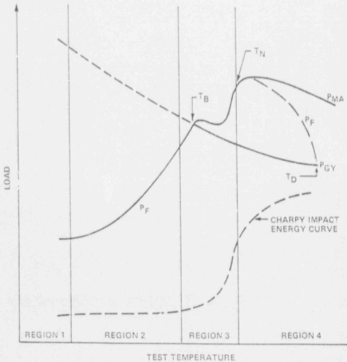
Figure III-3 Variation in Impact Load with Test Temperature for Instrumented Charpy Impact Tests
