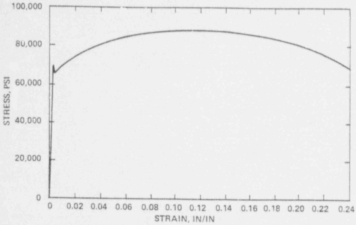
Figure VI-1: Stress-strain Record of Tensile Test
