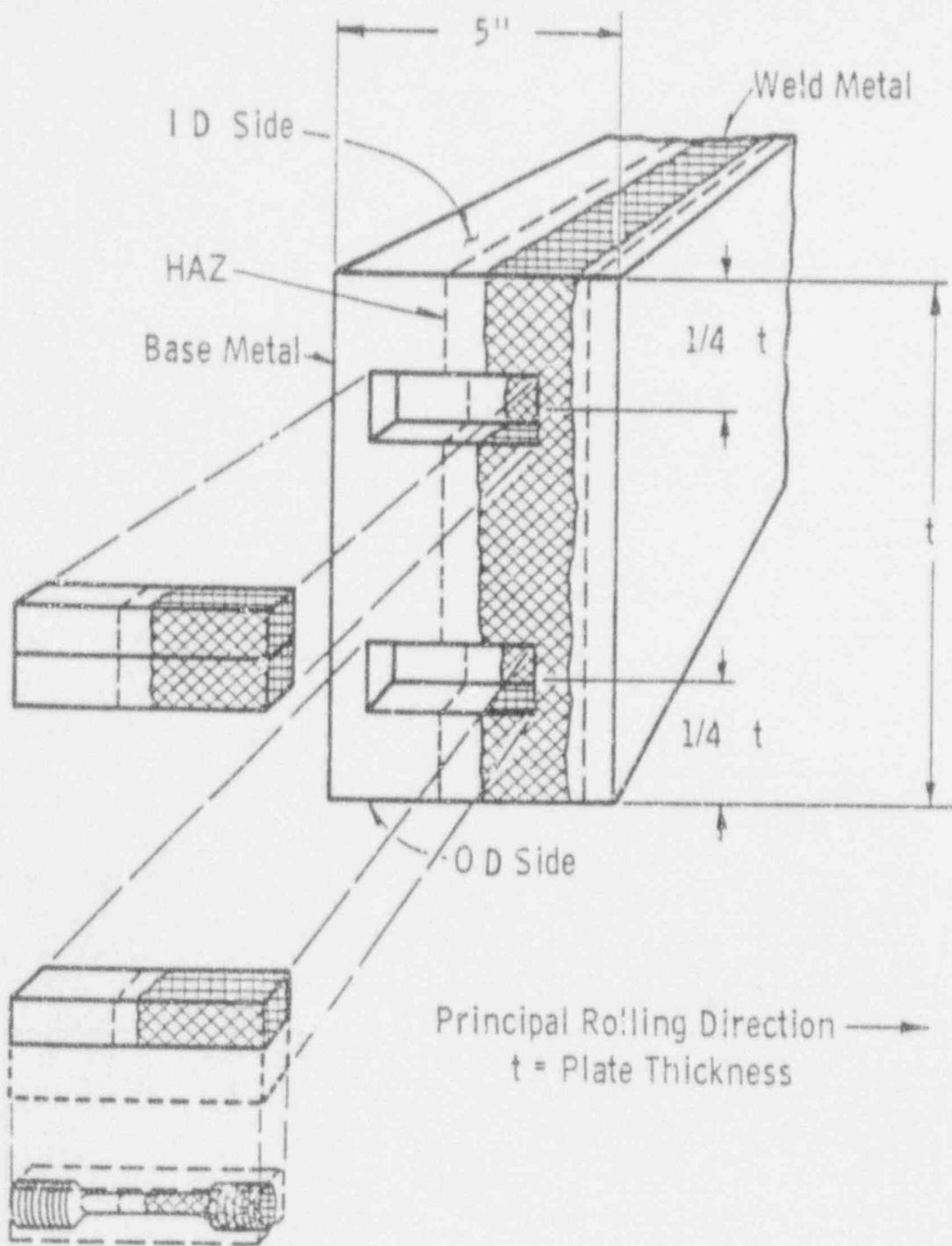
FIGURE: B-5. Location of Tensile Specimens
