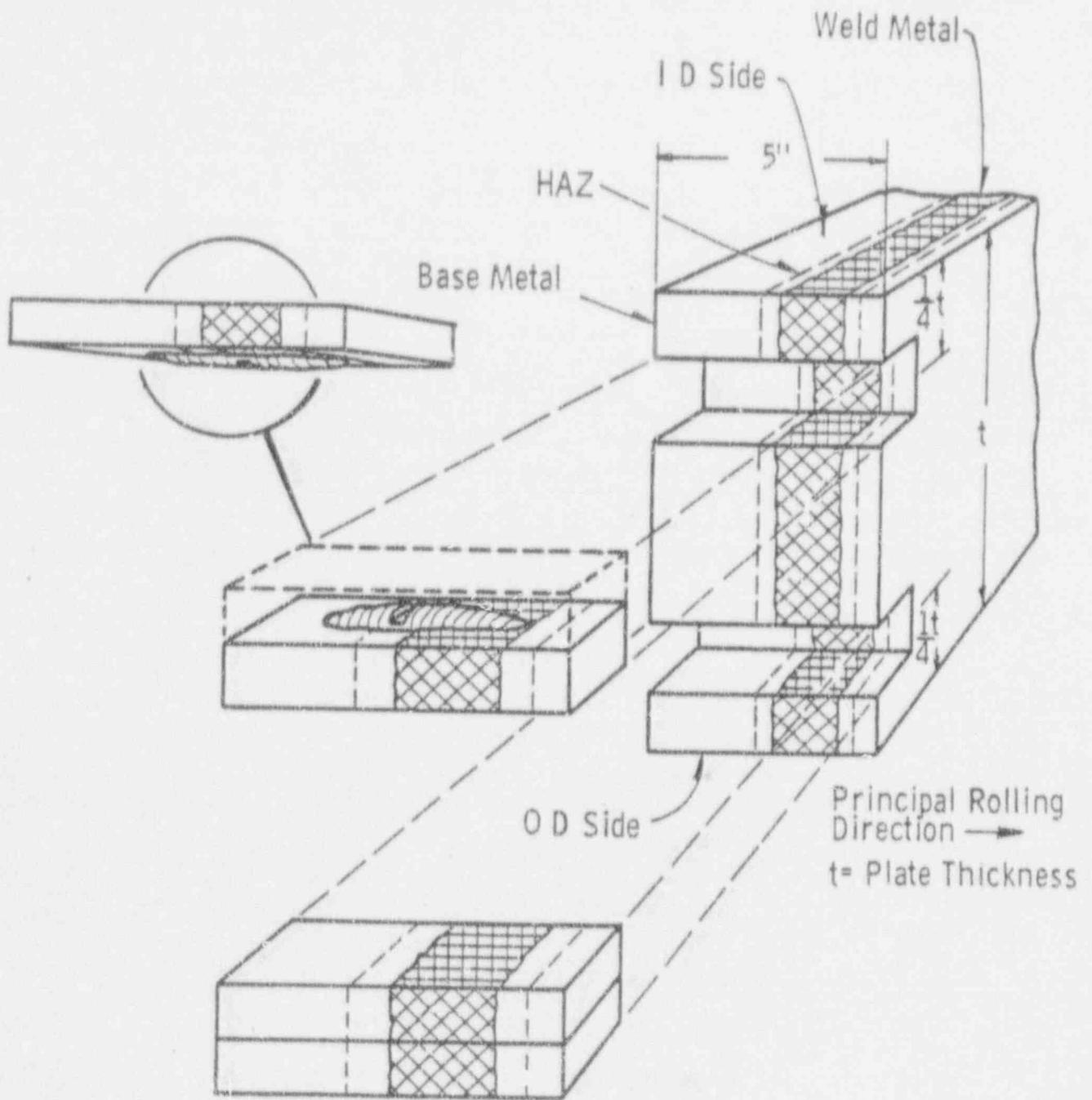
FIGURE: A-5. Location of Drop Weight Specimens Within Heat-Affected-Zone Test Material
