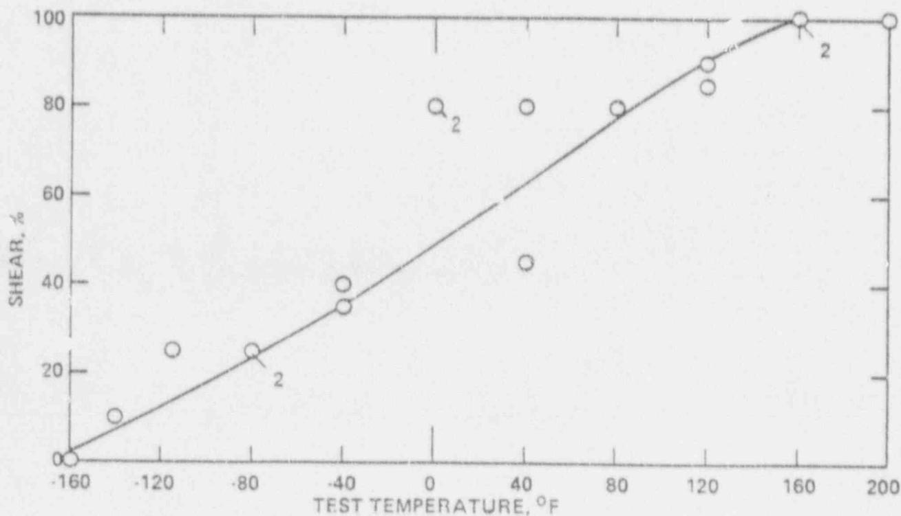
Figure VII-16: SHEAR vs TEMPERATURE
