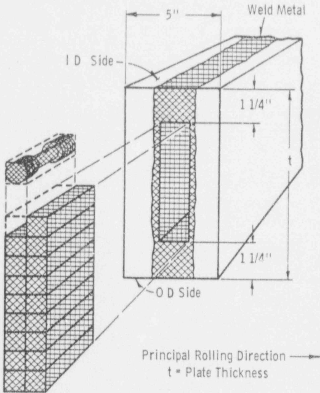
FIGURE: B-4. Location of Tensile Specimens
