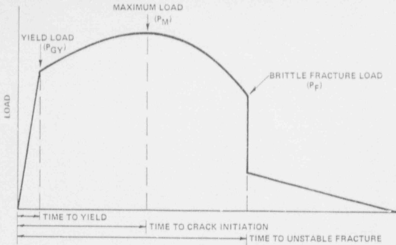
Figure III-1 Idealized Load - Time Record for Instrumented Impact Testing
