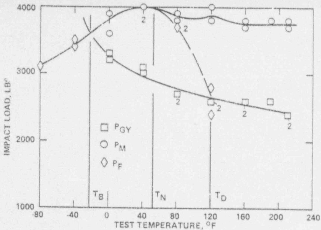
Figure VII-5: IMPACT LOAD vs TEMPERATURE
