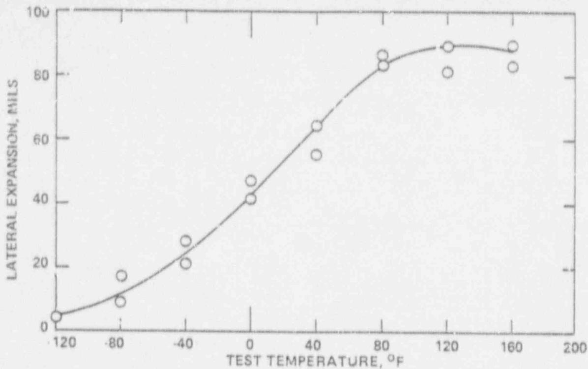
Figure VII-11: LATERAL EXPANSION vs TEMPERATURE
