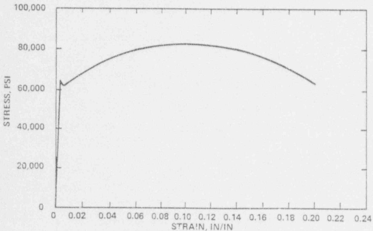
Figure VI-10: Stress-Strain Record of Tensile Test
