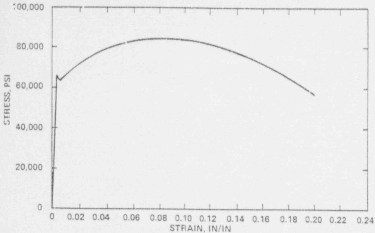
Figure VI-9: Stress-Strain Record of Tensile Test
