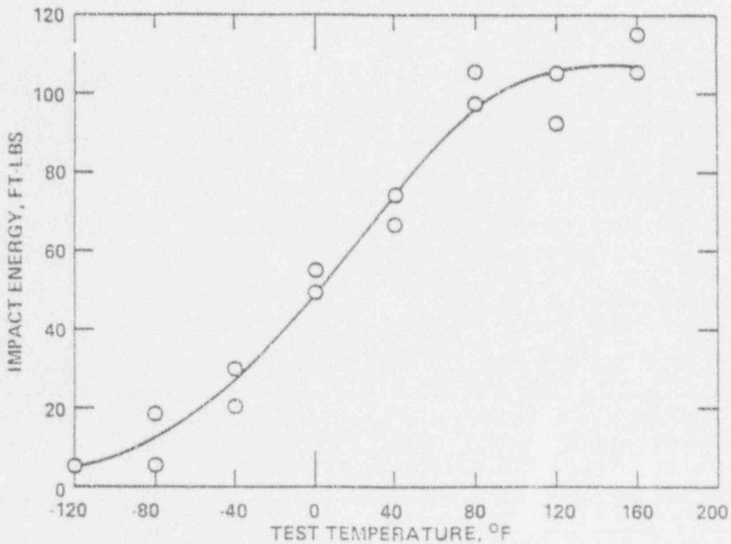
Figure VII-10: IMPACT ENERGY vs TEMPERATURE
