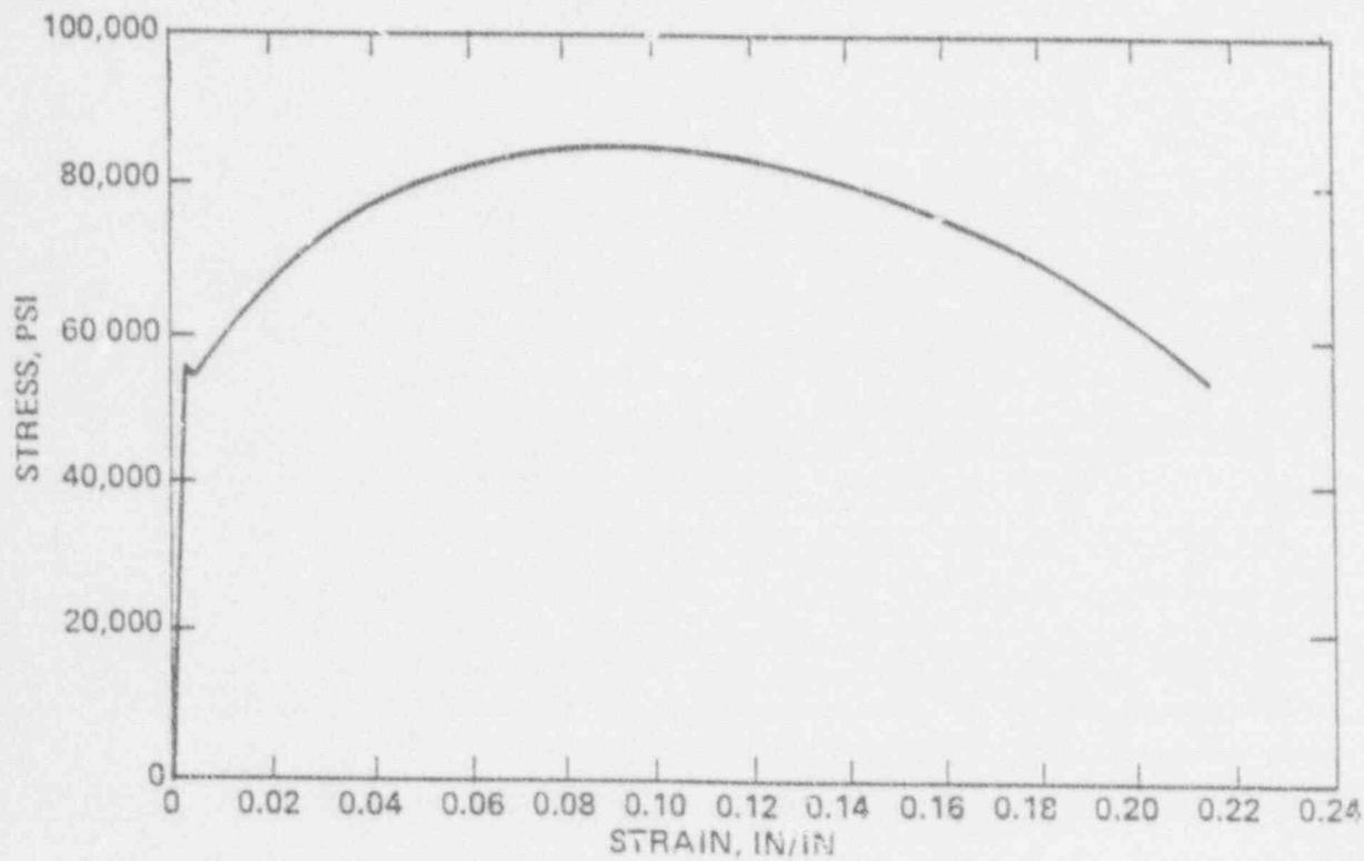
Figure VI-6: Stress-Strain Record of Tensile Test
