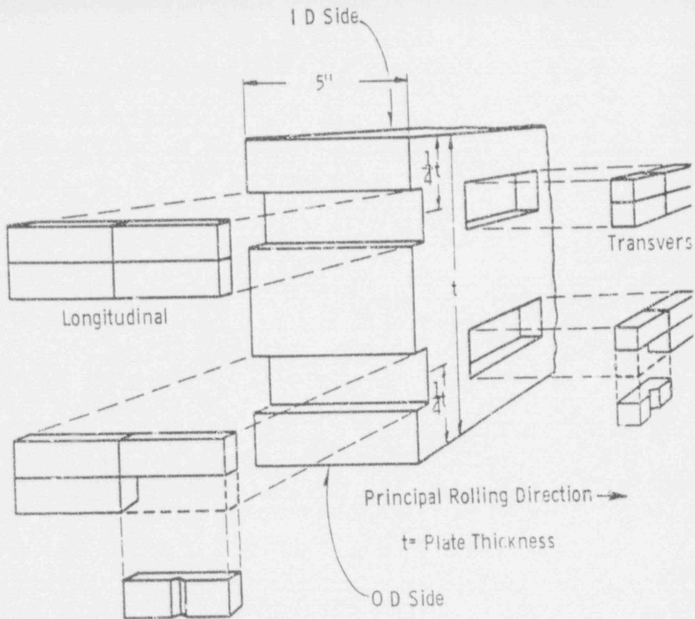
FIGURE: C-3. Location of Charpy Impact Specimens Within Base Metal Test Material
