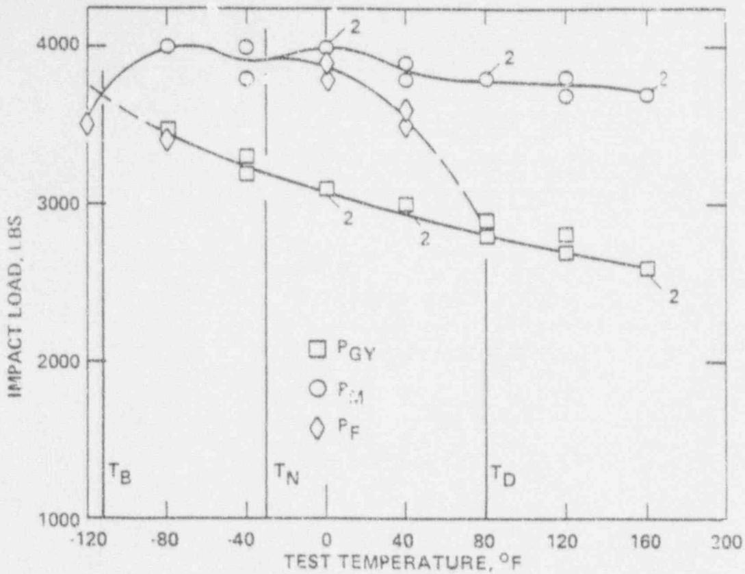
Figure VII-9: IMPACT LOAD vs TEMPERATURE
