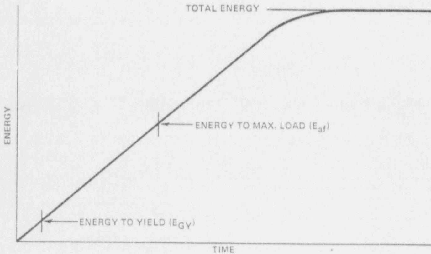
Figure III-2 Idealized Energy - Time Record for Instrumented Impact Testing
