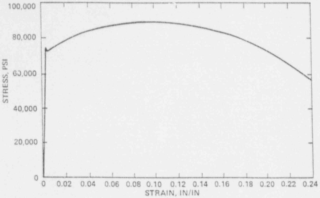
Figure VI-7: Stress-Strain Record of Tensile Test
