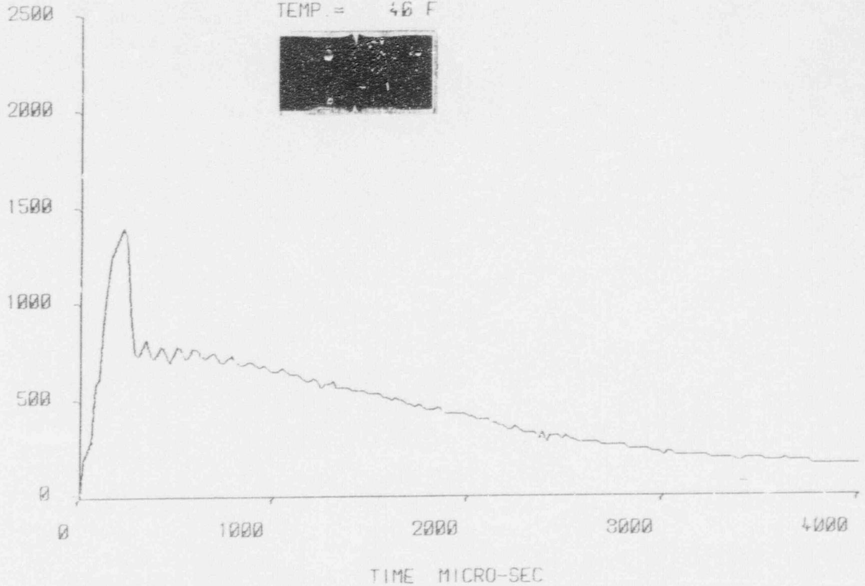
Figure VIII-4:  $PIC_V$  Load Record for Base Metal Plate D-4802-2 (WR)
