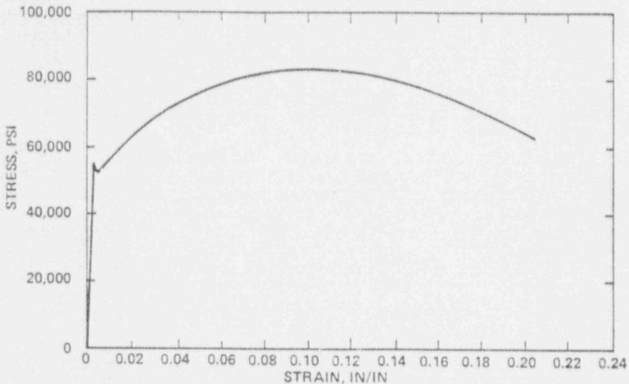
Figure VI-3: Stress-Strain Record of Tensile Test
