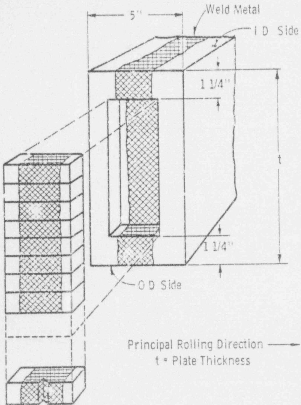
FIGURE: C-4. Location of Charpy Impact Specimens Within Weld Metal Test Material
