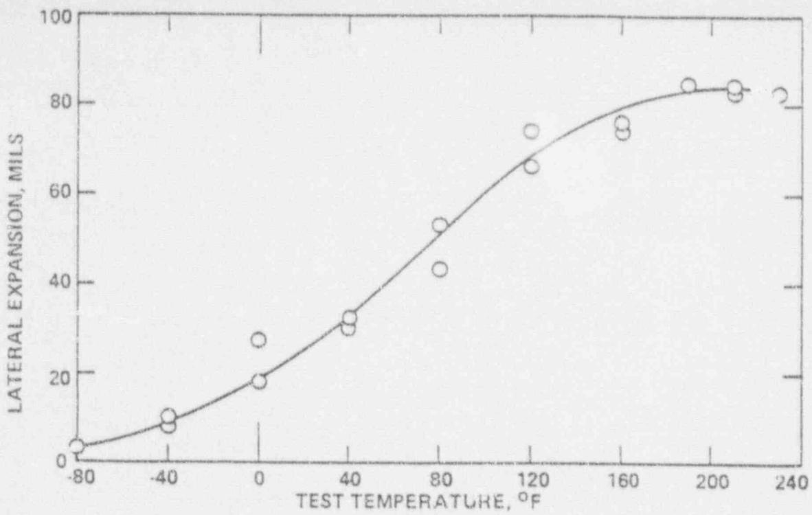
Figure VII-3: LATERAL EXPANSION vs TEMPERATURE
