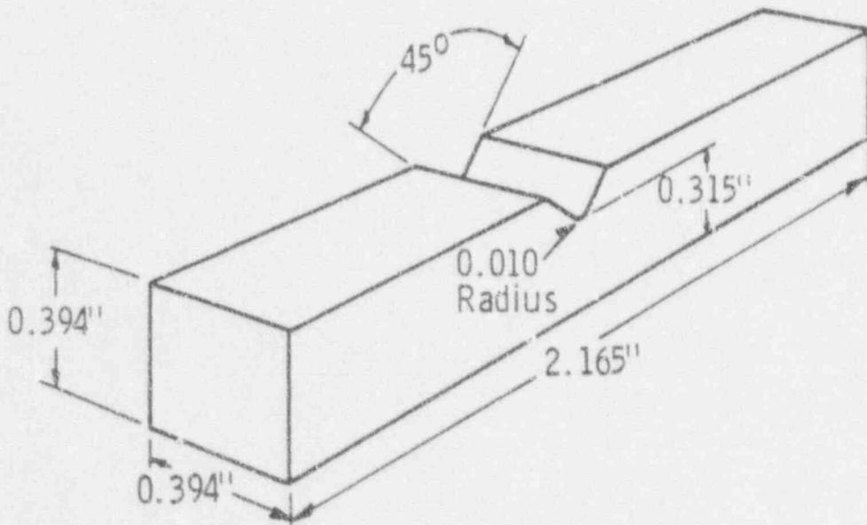
FIGURE: C-2. Typical Charpy V-Notch Impact Specimen
