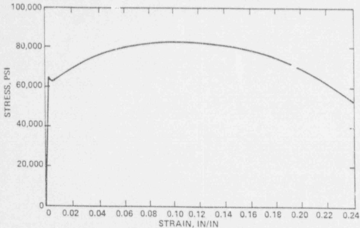
Figure VI-5: Stress-Strain Record of Tensile Test
