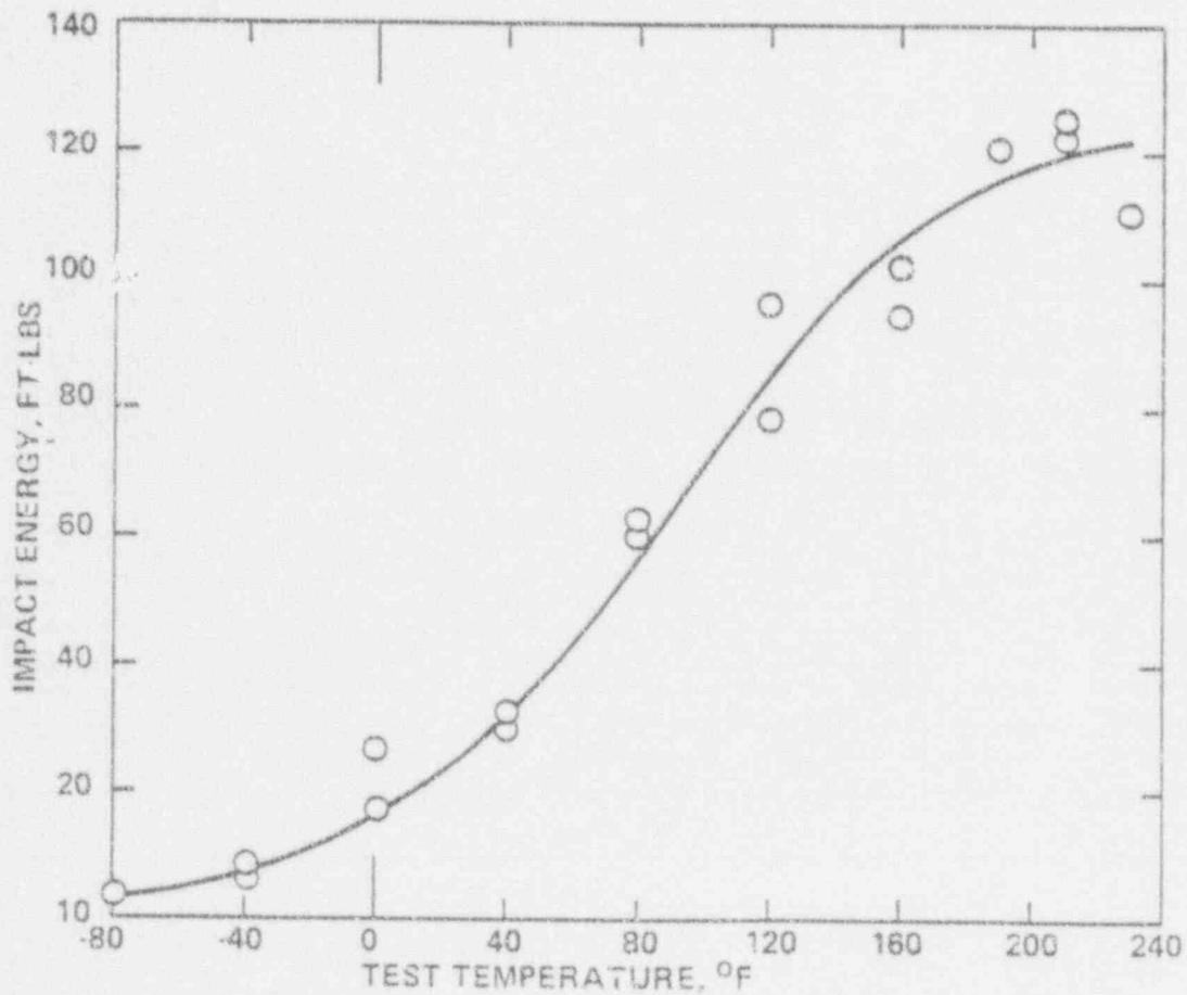
Figure VII-2: IMPACT ENERGY vs TEMPERATURE
