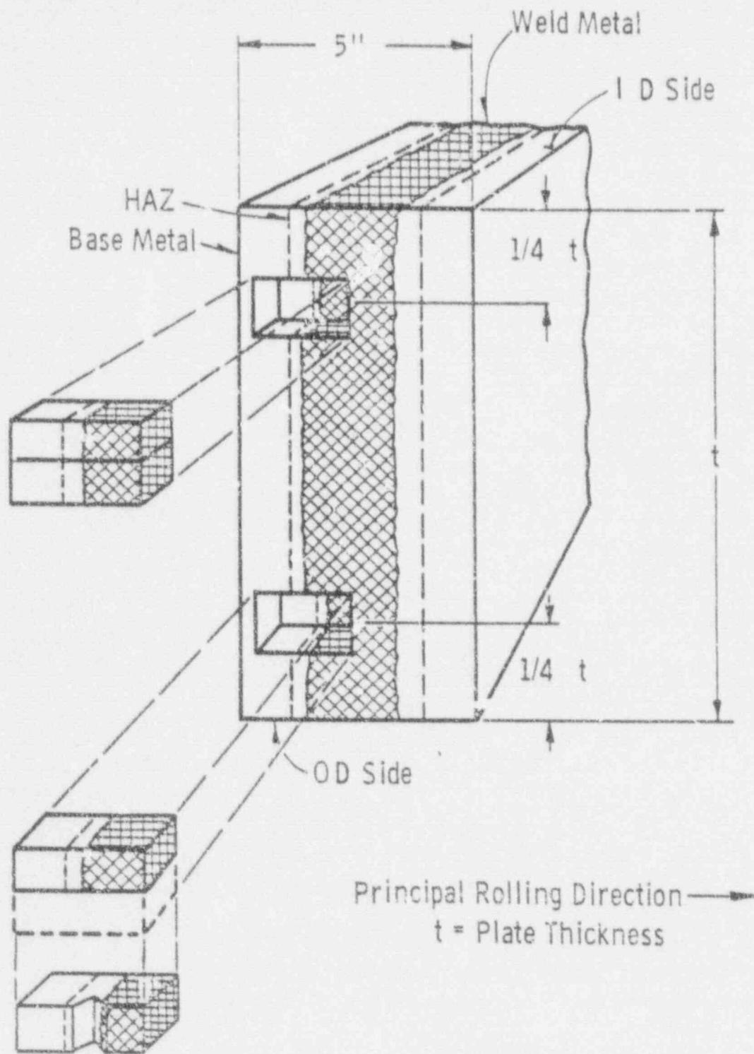
FIGURE: C-5. Location of Charpy Impact Specimens Within Heat-Affected-Zone Test Material
