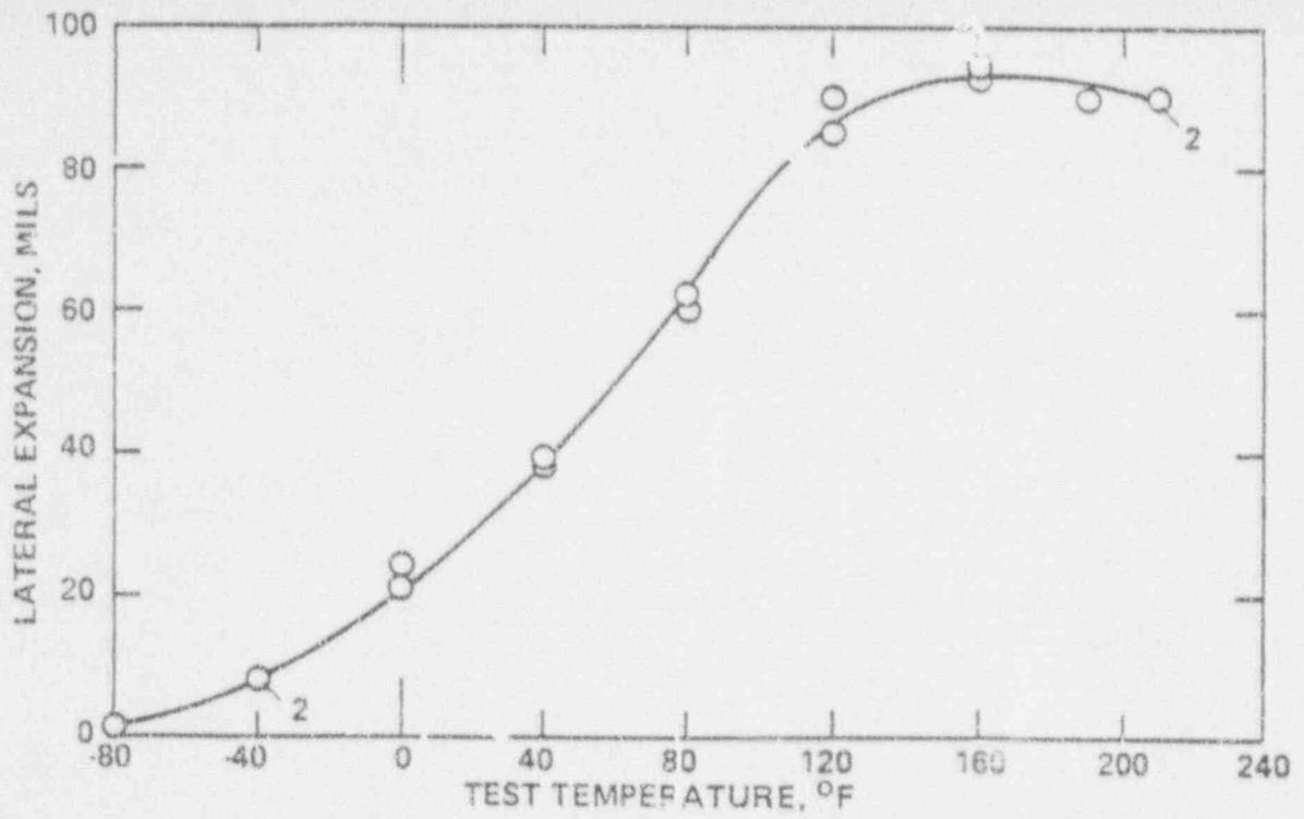
Figure VII-7: LATERAL EXPANSION vs TEMPERATURE
