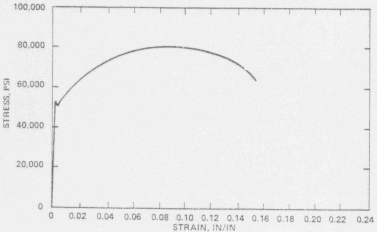
Figure VI-12: Stress-Strain Record of Tensile Test
