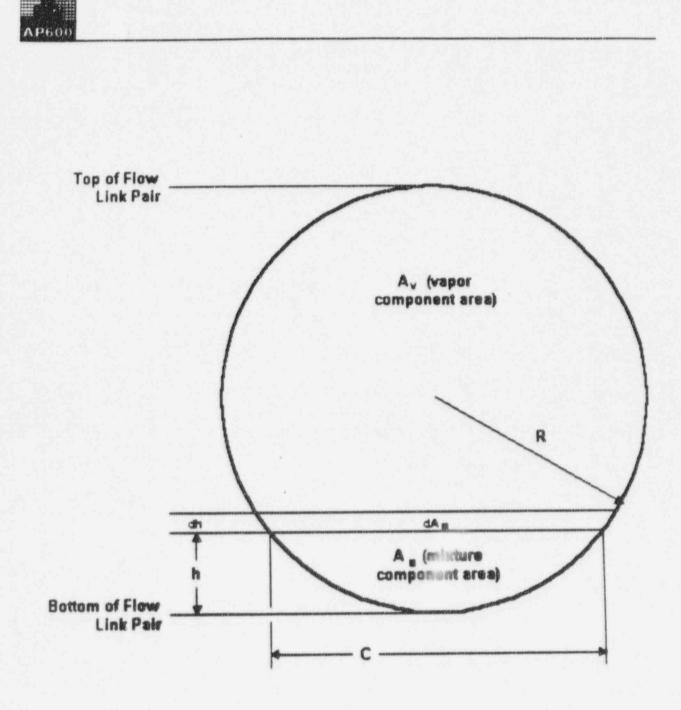
Figure 4.5-2 Cross-Section of Horizontally-Stratified Flow Link Pair
