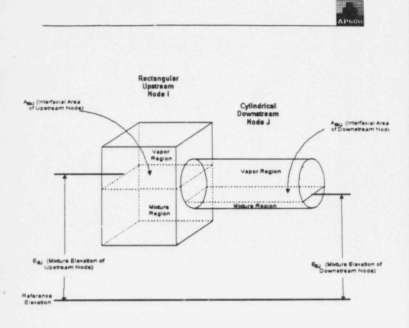
Figure 4.5-1 Geometry to Which the Horizontally Stratified Flow Link Pair Model Would Typically be Applied
