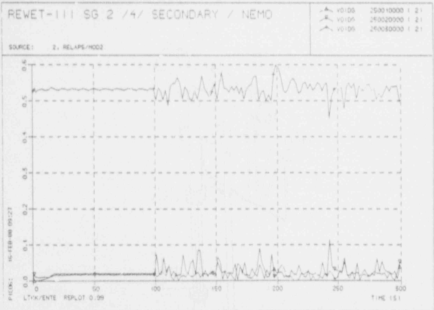
Fig. 14. Steam generator hydrodynamic instability appears when the requested time step is increased from 0.25 to 1.0 s. The Courant limit is about 0.7 s, and the code immediately resets the time step to 0.5 s.
