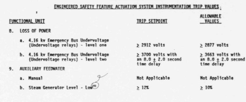
(1) For Cycle 12 only, OPERABILITY of the auxiliary feedwater (AFW) automatic initiation logic will rely on operator action to ensure successful initiation of AFW. Prior to startup for Cycle 13, modifications to the automatic initiation logic for AFW will be implemented to eliminate the reliance on operator action. 6/7/94
